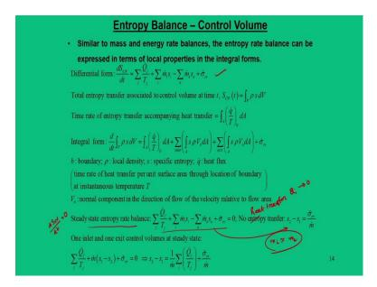
Now let us move more closely and this particular slide shows the elaborate version of this differential form of equations for the control volume and the simplified sense that this particular equation gets simplified for a steady state entropy rate balance.
