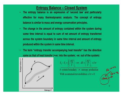
Now let us evaluate that particular equation in a more elaborate way; that means, here we have shown from initial state to final state it goes in an irreversible path and returns to a reversible path.
