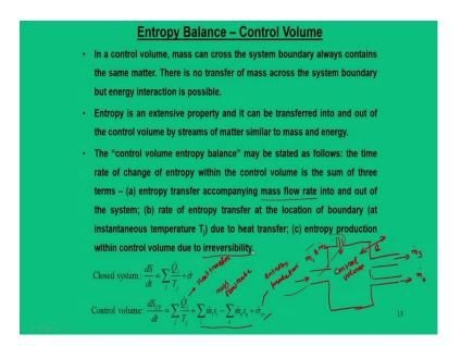
Now, let us move to entropy balance equations for the control volume. So, basic difference between a closed systems and control volume is that in a control volume, both mass and energy interaction is possible.
