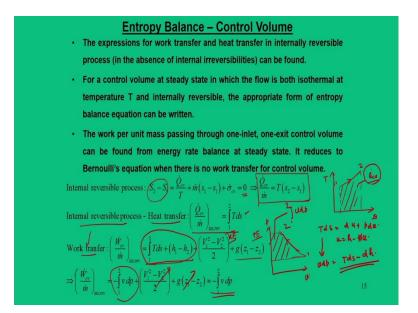
Now another aspect of entropy balance for the control volume is to elaborate the expressions of work transfer and heat transfer for the internal reversible processes.
