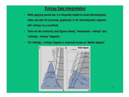
So, more clear pictures is shown here, the temperature entropy diagrams and enthalpy entropy diagrams. This enthalpy entropy diagrams we normally call this as a Mollier diagrams. So, you can see here, in this dome we have saturated liquid, we have saturated vapour and this is demarcated by the critical point  $c_{p}$ , similarly in the enthalpy entropy diagram or Mollier diagram.
