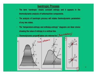
So, last segment of our discussion is about isentropic processes. So, the word isentropic process we mean it is a constant entropy process; that means, system undergoes change of state from one to two without involving in change of entropy.
