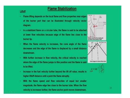
The next important aspect as I mentioned is that lift off. We except that burner that the flame should sit on the burner port it should not get lifted. To counter this argument if you see this particular figure here why the flame gets lift off and in fact, here also the same philosophy we say this is the half of this burner tube and where least gas velocity is 0, maximum is at the centerline velocity and the nature of the flame we can see through this profile.
