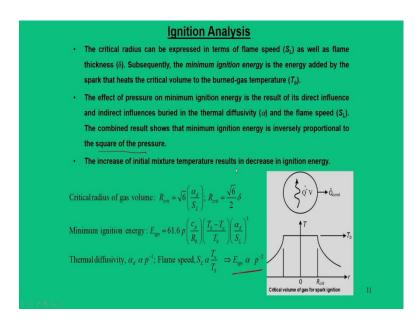
So, this gives a conclusion that we can find the critical radius and this critical radius can be expressed in terms of flame speed as well as the flame thickness delta, minimum ignition energy is the energy added by this spark that heats the critical volume to the burnt gas temperatures that is the minimum ignition energy.
