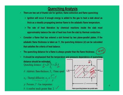
So, with this concept let us give some mathematical insight into the quenching distance. So, what we consider here? If you refer to this figure, we are looking at a flame that enters to the slot of diameter d and this flame has thickness  $\delta$ . So, this we say is a flame, now within this flame if you see this is the entire volume in which the flame is being produced.
