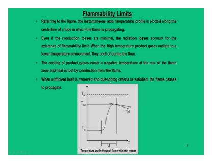
Now, after this we can clearly see there is a drop in the temperatures and that drop is mainly due to the issues that heat is lost by conductions from the flame. So, the cooling product gas create a negative temperature at the rear of the flame zones which means that heat is lost from this flame. When sufficient heat is removed the quenching criteria is satisfied. So, flame chooses to propagate; that means flame does not move further.
