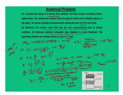
So, this gives mixture mass flow rate per unit cross sectional area. The second part is we need to find the maximum allowable tube diameter, for that we recall our relations
