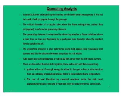
So, let us start the first thing which is called as quenching analysis. So, the first parameter of flame extinguishing is the quenching. So, in general flames extinguish upon entering sufficiently small passage way and if it is not too small the flame will propagate further.
