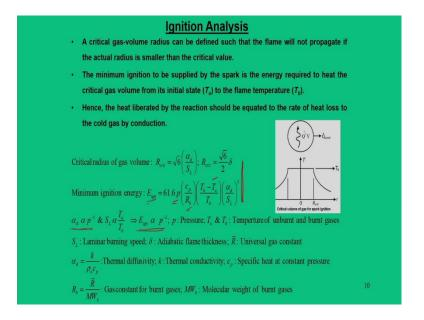
So, what we are looking at is that by creating this spark whether we are able to give sufficient energy or not. So, to do that we can find a critical gas volume radius which can be defined such that, flame will propagate if actual radius is smaller than the critical value. So, in other words; that means, for a flame propagating situation; that means, it has enough energy in it so, that it can propagate further and at the same time there is a heat loss from the flame through the conductions.
