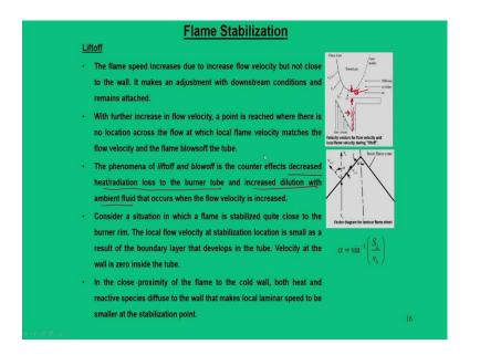
So; that means, subsequent increase in the flame velocity will make the flame to its best possible extent to adjust with respect to downstream conditions, because there are two counter effects when it gets lift off. One is decreased heat radiation loss to the burner tube, other is increased dilution with respect to ambient fluid, because the ambient fluid tries to enter through this lift off distance.
