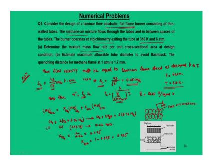
Now, with this we are now in a position to discuss some numerical problems what we have understood so far. The first problem is about the design of a laminar adiabatic flame burner and we expect that we need to have a flat flame; it consists of thin-walled tubes. So, if you recall our one of the pictures this is a case for an adiabatic fuel burner, in which fuel air mixture comes through it and we have some glass balls or some regions or you can say they are pre heated zones.
