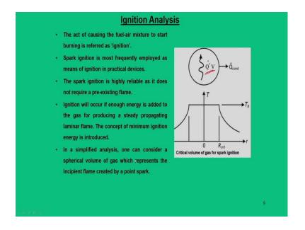
Next important topic of discussion is the ignition. So, the act of causing fuel and air mixture to start burning is referred as the ignition and in particular we normally refer with respect to spark. We know that in a engine spark ignition engines that is a spark plug through which we ignite the fuel.
