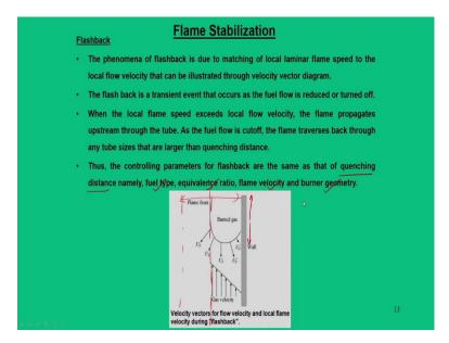
Now, let us understand one by one why the flash back has to occur. So, why it occurs that is because if you look at actually flash back how it happens that there are two speeds that controls the motion of the flame. First is flame speed at which the flame moves ahead and there is the gas velocity that pushes the flame further. And these two things allows that we have a steady flow laminar flame, but when there is a mismatch between the local laminar speed to the local flow velocity.
