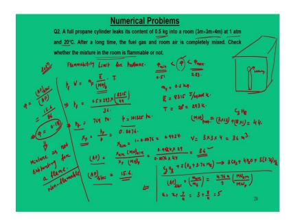
And the second problem is about the flammability limit. So, what we have is that a full propane cylinder it is there in a room it contains 0.5 kg. The room size is 3 meter into 3 meter into 4 meter and room condition is 1 atmosphere and 20 C. So, after a long time the fuel and room air is completely mixed. So, we have a room in which we have a gas cylinder, gas is leaking.
