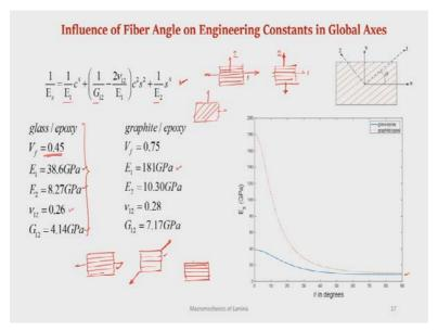
Using the expression of  $E_x$  in terms of  $E_1$ ,  $E_2$ ,  $G_{12}$ ,  $v_{12}$  and  $\theta$ ,  $E_x$  has been plotted for different values of  $\theta$  between  $0^{\circ}$  to  $90^{\circ}$ , for two kinds of lamina viz. glass epoxy for a volume fraction of 45% and a graphite epoxy for a volume fraction of 75% as shown in Fig.
