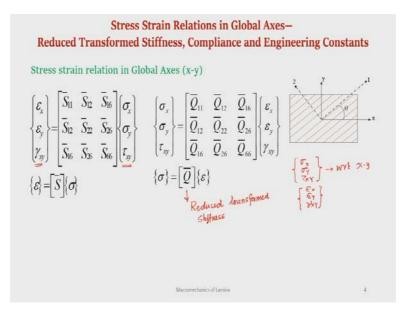
Then, we have also used our knowledge of stress and strain transformation and we could actually obtain the relations between the stresses and strains in the global axes. That means, the stresses and strains with respect to x-y. This stress is with respect to the Cartesian coordinate axes x-y; and similarly, the corresponding strains,  $\varepsilon_x$ ,  $\varepsilon_y$ ,  $\gamma_{xy}$ . And we have obtained the relationship; how did we do so?
