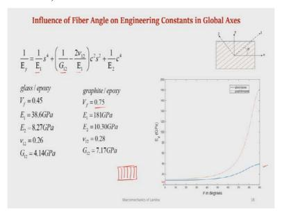
Similarly, we can see the variation of  $E_y$ , at  $\theta = 0^\circ$ ,  $E_y = E_2$ , at  $\theta = 90^\circ$ ,  $E_y = E_1$ ; and in between, it varies. Figure shows the variation of  $E_y$  for glass epoxy and graphite epoxy.
