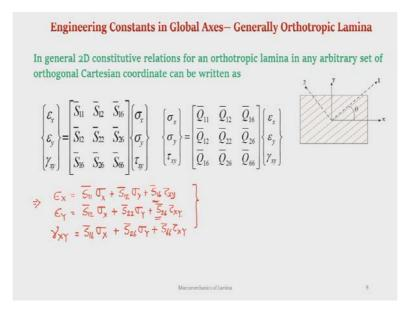
Now, having understood this stress-strain relationship using reduced transformed stiffness and transformed compliance matrix, let us try to understand the engineering constants with reference to x-y axes for a generally orthotropic angle lamina.
