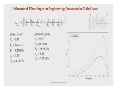
Similarly, we could plot the variation of  $\eta_{xy,y}$  with  $\theta$  using the expression in terms of  $E_1$ ,  $E_2$ ,  $G_{12}$  and  $v_{12}$ . Again, for be 0 at  $\theta = 0^{\circ}$  and  $\theta = 90^{\circ}$  the value is zero and it is maximum value and the corresponding at  $\theta$  at which it is maximum depends upon the values of  $E_1$ ,  $E_2$ ,  $G_{12}$  and  $v_{12}$ .
