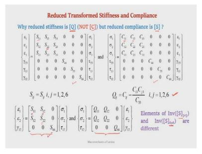
Now, just before we actually go to the engineering constants for a generally orthotropic lamina, just a note that many a times this question comes, the reduced stiffness matrix is actually, or reduced transformed stiffness matrix is actually denoted by Q, not by C; whereas the compliance is S. If you remember, for an orthotropic or in general, for 3-dimensional, the compliance matrix is always denoted by S and the stiffness is by C.
