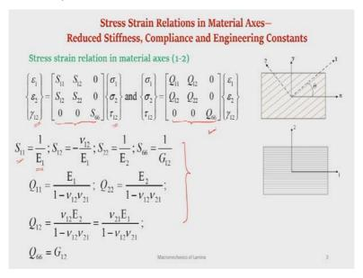
Then, we have developed the stress-strain relationship wherein suppose the stresses in the material axes are related to the corresponding strains and this is the compliance matrix and this is the reduced stiffness matrix; I think we have discussed these things in details in the last class. And then, we could relate the engineering constants in terms of, we could write engineering constant in terms of the elements of the compliance matrix and stiffness matrix like this; that we understood.
