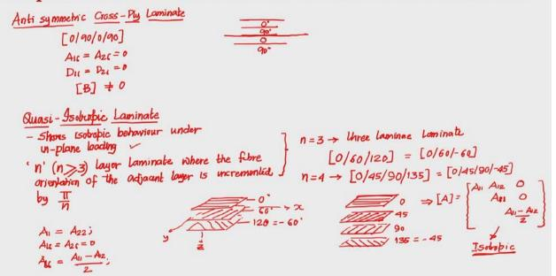
Similarly there could be anti-symmetric cross ply laminate. Like symmetric cross ply here also each ply is a specially orthotropic plies but for each 0° ply above the mid surface there is 90° symmetrically placed below the mid surface. For example, [0/90/0/90] an anti-symmetric cross ply laminate. So,
