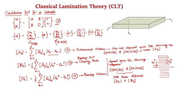
In the last lecture, the assumptions made in classical lamination theory and their significance was discussed in details. Key assumptions were assumptions on the nature of the displacement field, assumptions on strain displacement relationship, assumption on stress-strain relationship. Based on those assumptions the laminate constitutive equation was developed, where the force
