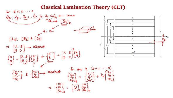
From the properties of each lamina we can determine the reduced stiffness matrix for each lamina as
