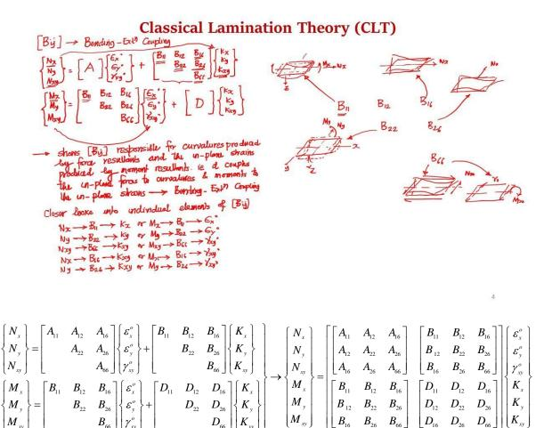
So, [A] is extensional matrix and within [A] matrix there coupling, and note that these are lamina coupling. Then [D] is the bending matrix, but within that [D] matrix there may be coupling. [B] is the coupling matrix that couples the in-plane forces to the curvatures and the moments to the implant strains.
