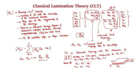
So, this [B] matrix which is the bending extension coupling has nothing to do with the anisotropy of the constituent lamina. It is only due to the un-symmetry of the stacking. Even in
