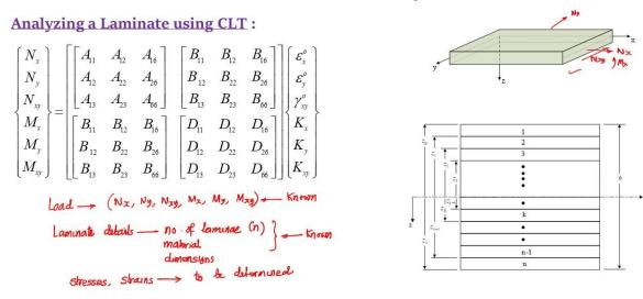
In general, the applied load on the laminate is known and the laminate details like the number of layers, material properties of each layer, fiber orientation of each layer, thickness of each layer, their locations, that is the stacking sequence are known. The stresses and strains need to be determined using CLT. This is as follows.
