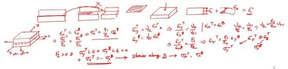
This knowledge of macromechanical analysis of lamina and micromechanical analysis of lamina, the stress strain behaviour of unidirectional for specially orthotropic or for angle lamina (where the material axis are oriented differently with respect to analysis axis or global axis) and the strength failure theories for such lamina are actually combined to establish the average stiffness or the response of a laminate under loading in classical lamination theory.
