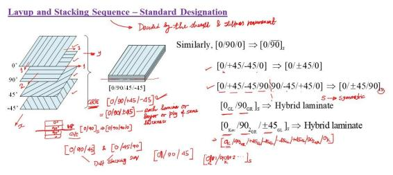
Let us first understand how a laminate is actually designated or specified. There are standard way of designating a laminate layup and stacking sequence. If four laminae say made of graphite/epoxy with fiber orientations  $0^{\circ}$ ,  $90^{\circ}$ ,  $+45^{\circ}$ ,  $-45^{\circ}$  are stacked together, then it is designated as  $[0^{\circ}/90^{\circ}/+45^{\circ}/-45^{\circ}]$  graphite/epoxy (GR/E) laminate. Again say
