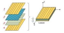
As shown in the Fig., there are 4 laminae stacked together to form a laminate and they are perfectly bonded, so as to act as one unit. A lamina is very thin and therefore to provide moderate thickness we stack several of them together to form a laminate. To understand why a laminate is actually required, let us revisit some of the important aspect of lamina what was discussed in micro and macromechanics of lamina.
