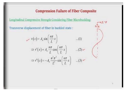
Now considering the fiber buckling, suppose considering the transverse displacement of the fiber to be sinusoidal (ref Fig.). The displacement along x is u and the displacement along y is v. The transverse displacement v is expressed as
