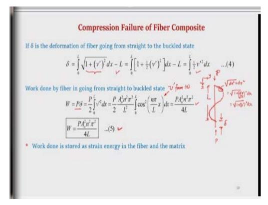
Considering a fiber which is initially straight and subjected to axial compression the axial deformation along  $x \delta$ . Suppose the length is *L* after it buckles, so the initial length is given by
