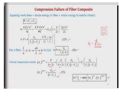
And now again equating the work done to the strain energies stored in the fiber (bending) and in the matrix (shear),
