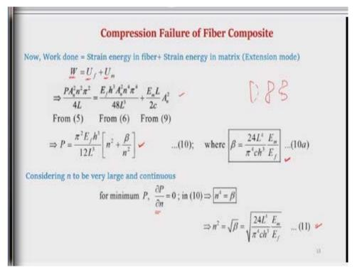
Now we have the work done from equation number (5), we have the strain energy stored in the fiber from equation number (6), strain energy stored in the matrix because of extension from equation number (9). Equating the work done to the strain energy stored as
