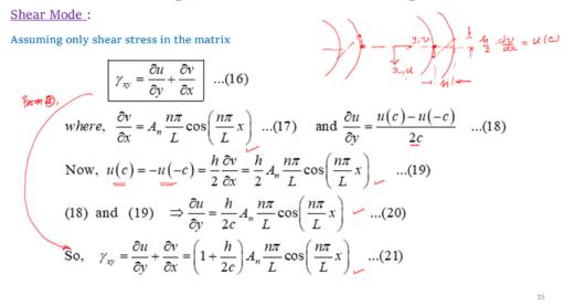
Referring to the Fig., in shear mode two adjacent fibers, separated by a distance 2c actually slide over each other. Therefore under shear, the points on the fibers move along x- direction (as shown)
