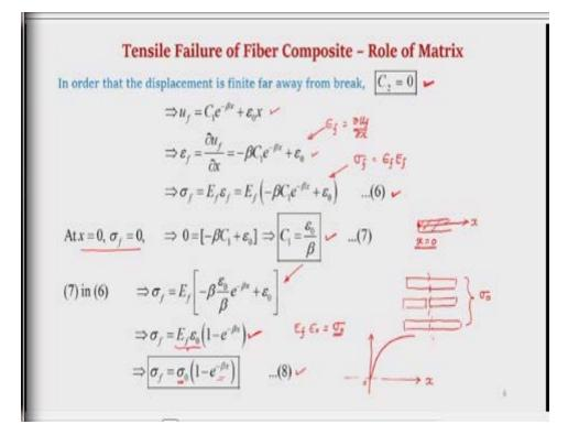
That means in order to ensure that the displacement is finite,  $C_2=0$  otherwise we get a solution which is not feasible. Therefore (7) gives
