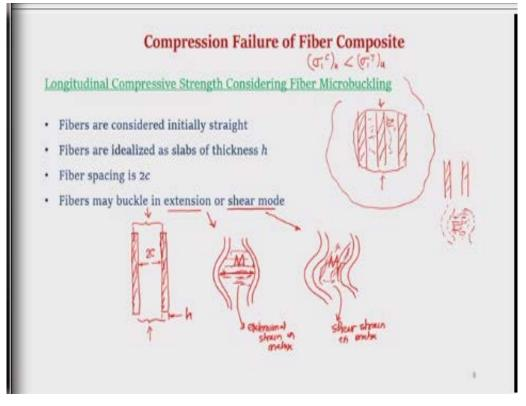
Next we will discuss the longitudinal compression of fiber composite considering fiber microbuckling. The longitudinal compression strength of fiber composite is much less compared to it is tensile strength and one of the reason is that the fibers are slender and therefore even though the composite as a whole does not buckle there may be fiber microbuckling.
