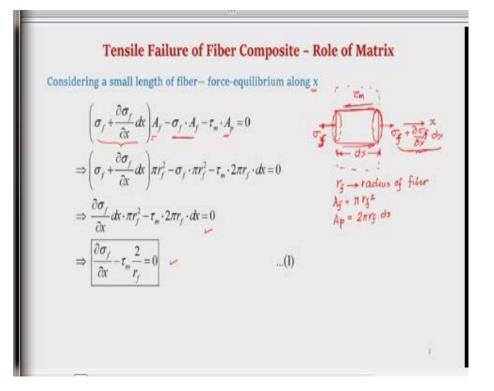
Considering a small length of the fiber, say dx. Because of the tensile load this is experiencing a
