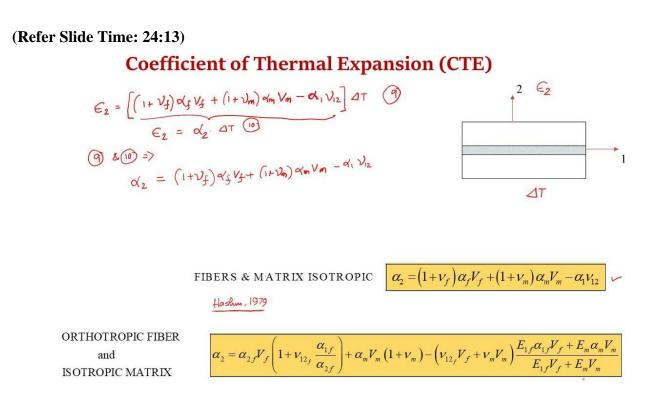
Now in deriving these expressions actually the both fiber and the matrix properties are isotropic. There are works (Hashin in 1979) where the properties of the fiber have been actually considered as orthotropic and the expression for  $\alpha_2$  is obtained as
