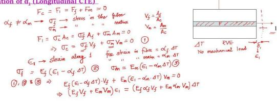
In this lecture, we will discuss the determination of coefficients of thermal expansion and coefficients of moisture expansion, the parameters responsible for hygrothermal response of a lamina. The importance of the determination of hygrothermal stresses in a lamina was already discussed while discussing the hygrothermal stresses in lamina.
