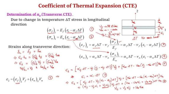
Here also the same RVE is considered as shown only subjected to  $\Delta T$ , no mechanical load. When this RVE of the composite actually experiences a temperature changes of  $\Delta T$ , the strain in this direction is  $\varepsilon_1$  and because of the perfect bonding, the fiber, the matrix and the composite experiences the same strain along 1.
