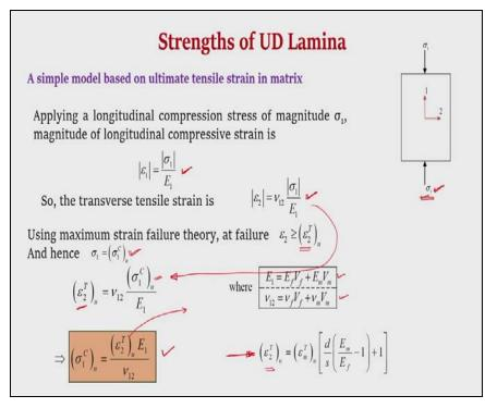
Next is a longitudinal compressive strength of a composite. Now the models which are actually used for tensile strength may not be suitable for longitudinal compressive strength. Because under compression the failure modes are different there are different possible failure modes like transverse tensile, shear failure, fiber micro buckling.
