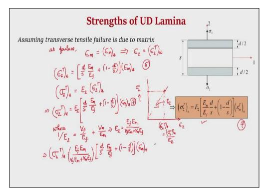
Now with the assumption that the transverse failure of the composite is due to the failure of the matrix meaning that at failure, the strain in the matrix  $\varepsilon_m$  is equal to ultimate strength of the matrix. So, from the last equation that means equation number 5 we can now write we can replace  $\varepsilon_m$  by  $(\varepsilon_m)_u$  and  $\varepsilon_2$  as  $(\varepsilon_2^T)_u$ .
