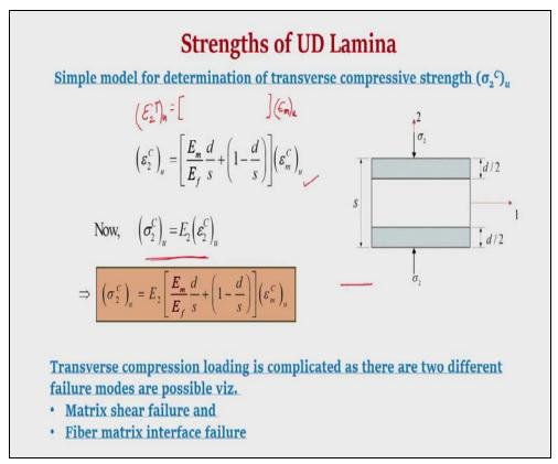
Next let us discuss the determination of transverse compressive strength. So, again a simple model analogous to the transverse tensile strength could be used. It is similar to transverse tensile strength but we have replaced the tension by compression and the same expression which was derived for the transverse tensile strength is used where  $(\varepsilon_2^T)_u$  is replaced by  $(\varepsilon_2^C)_u$  and  $(\varepsilon_m)_u$  is replaced by  $(\varepsilon_m^C)_u$  in the following expression
