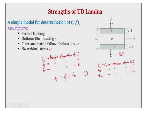
In the last lecture, longitudinal tensile strength of a lamina was discussed. Now, let us discuss the transverse tensile strength. Unlike the longitudinal tensile strength which is almost entirely decided by the fiber properties, the transverse tensile strength is actually influenced by many other factors like bond strength of the interface presence of voids etc.
