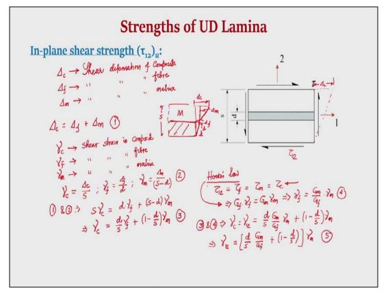
Next let us discuss the in plane shear strength. Again as shown in the Fig. considering an subjected to pure shear it is subjected to pure shear  $\tau_{12}$ . Now, suppose  $\Delta_c$ ,  $\Delta_f$  and  $\Delta_m$  are the shear deformation of the composite, fiber and the matrix respectively due to  $\tau_{12}$ . Therefore
