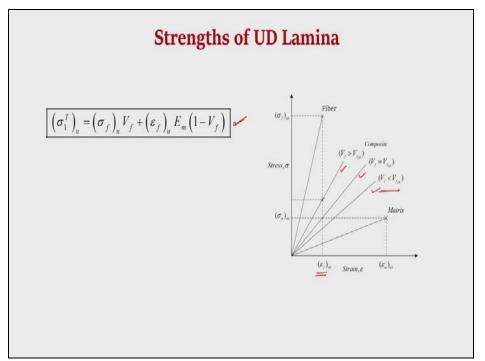
So, when the fibers fail that means when the strain in the fiber reaches the ultimate strain of the fiber then the composite fails and based on that an expression for the longitudinal tensile strength of the composite was derived which is dependent on the strengths and stiffness properties of the fiber and matrix and volume fraction. Therefore, for a given combination of fiber and matrix and for given properties of the fibers and the matrix is the volume fraction
