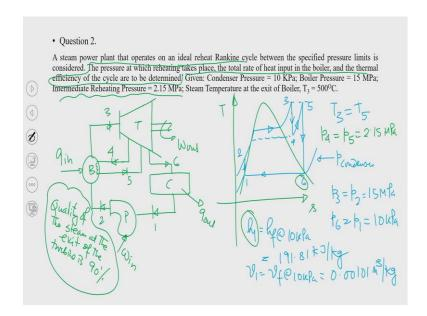
So, the next problem is a steam power plant that operates on an ideal reheat Rankine cycle between the specified pressure limits. The pressure at which reheating takes place, the total rate of heat input to the boiler, and thermal efficiency of the cycle have to be determined.
