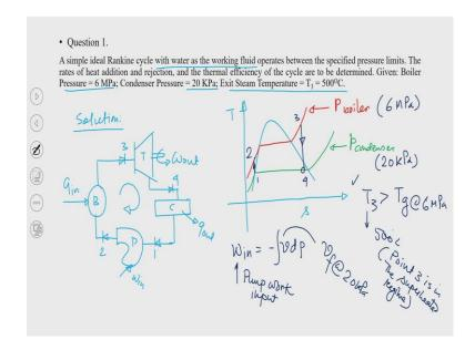
So, illustrating this numerical problem. We shall see that in practical scenario, when a steam power plant is operated then, what will be the maximum efficiency that we can expect. Not only that, we will see that water is allowed to go into the boiler, wherein
