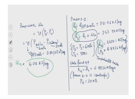
So,  $w_{in} = \int v dp = v \left( p_2 - p_1 \right)$ . So, sole objective of having this pump in this plant is to rise pressure from 1 to 2. So, pressure is increasing from  $p_1$  to  $p_2$ . So,  $p_1$  is nothing but  $p_{condenser}$  and  $p_2$  is nothing but  $p_{boiler}$ . So, this is  $w_{in} = v_f \Big|_{20kpa} \left( p_{boiler} - p_{condenser} \right)$ . Point 1 is lying on the saturated liquid line, and hence,  $v_i$  should be  $v_i$  at 20 kpa.
