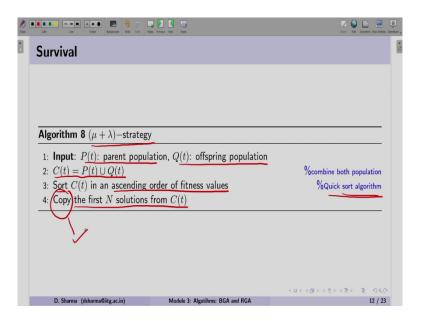
Now, come to the survival stage; this is we know it is the last function or implementation that is required for BGA to work. Now, in this case, you can see algorithm 8 is developed using mu plus lambda strategy.
