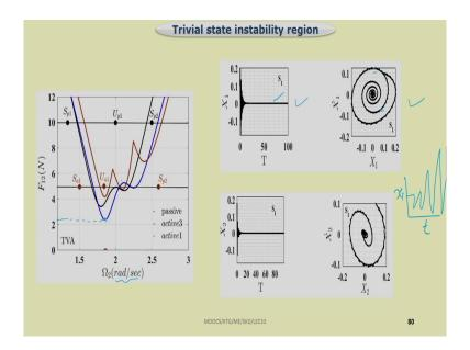
So at a different position, so you can plot the response plot also. So by plotting this response you can see the system to be the you can study the stability of the system. So for example, here it is written so here we have found the response at the stable point so you can see in phase portrait and in so this is the phase portrait plotted and this is the time response X 1 versus T is plotted.
