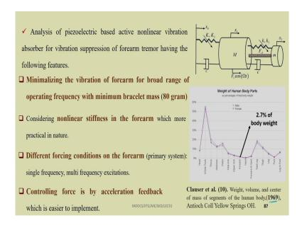
So, to control the vibration of the system one can use a bracelet so in the forearm one can use a bracelet having these effective mass and spring conditions and then it can be studied. So, you just see while designing such a system analysis of piezoelectric based active non-linear vibration absorber can be used for the suppression of the tremor in the hand using the following features.
