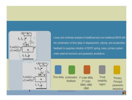
So, this work is part of the PhD thesis of Mr. Sibananda Mohanty, who is working under my guidance. Here, let us see this linear and non-linear analysis of traditional and non traditional active non-linear vibration absorber with combination of time delay in displacement, velocity and acceleration feedback to suppress the vibration of single degree of freedom spring, mass, primary system under external harmonic and parametric excitation.
