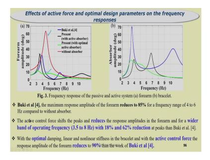
So, here the response become unstable. If we are using this effect of active force and optimal design parameter in the frequency response, so you can observe that for a wide range so it can be observed for that for a wide range we can control the maximum or peak amplitude.
