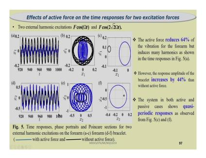
So, response amplitude clearly you can see so it is reducing significantly. So the active force produces 64 percent of the vibration of the forearm, but induces many harmonics as shown in this figure so it reduces many harmonics.
