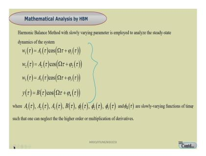
Then you can either use this method of multiple scale or use these harmonic balance method so here harmonic balance method is used.
