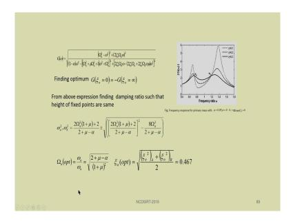
Similarly, here we can by using this transfer function. So we can write down these equations of the transfer from the transfer function we can find this thing G omega so that is the response amplitude so versus this response amplitude versus the frequency ratio. One can plot and find the value of these omega a omega b at which irrespective of damping so it is having the same value of response amplitude.
