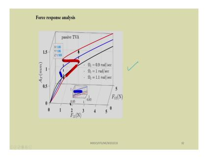
So, you can plot the force response plot also so for example, so you can take this F 11 2, you can vary this forcing F 11, F 12, simultaneously and see what will happen to this response amplitude in a 3D plot you can plot these thing and you can verify the response. So this way you can verify the system.
