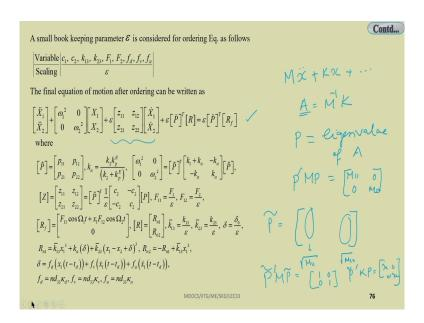
Here, by using a small book keeping parameter and ordering this equation of different order of scaling for example, the c 1, c 2, k 13 k, 23, F 1, F 2, f d, f b and f a are taken as order of epsilon.
