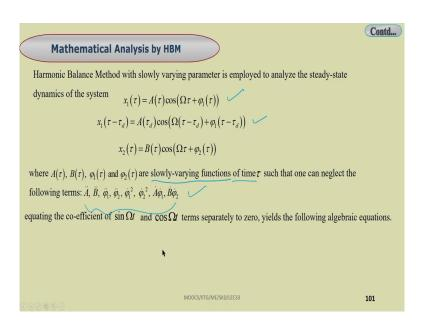
So, taking different system parameter. Previously, we have used this method of multiple scales. So here, I am showing you how you can use this harmonic balance method to solve similar system. So when you are applying this harmonic balance method, so you can take many terms or you can consider this way also.
