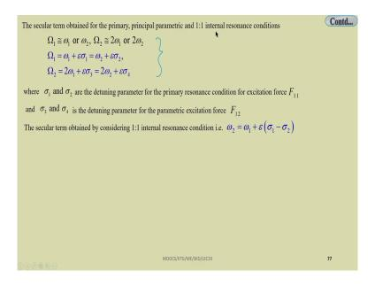
So, you can see, so there are different resonance conditions will be there the resonance conditions. For example, so you can had omega or you can have omega 1 equal to omega 1 that is external frequency capital omega 1; capital omega 1 is for the direct forcing. So, omega 1 equal to nearly equal to omega 1 or omega 2.
