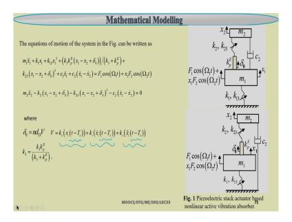
So after deriving this equation of motion, so you can see so how we can give the time delay to the system. So here we are considering a time delays; that means, whenever we are applying this force it will take some time to react, that is why there is a time delay in the response term.
