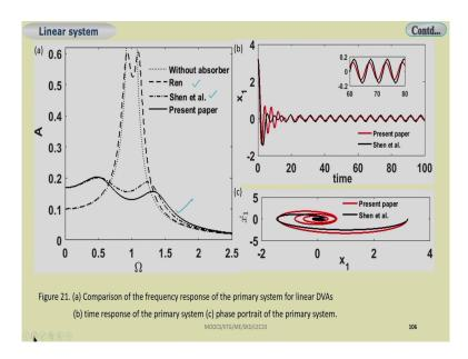
So, now by you can see the response so without absorber so it is comparison is given here. So you just see this curve is without absorber so if damping is considered. So you have two equal peaks here. So, now these two are by other two different researcher and in the present case by considering properly the system parameter, so you can observe that it is reduced significantly.
