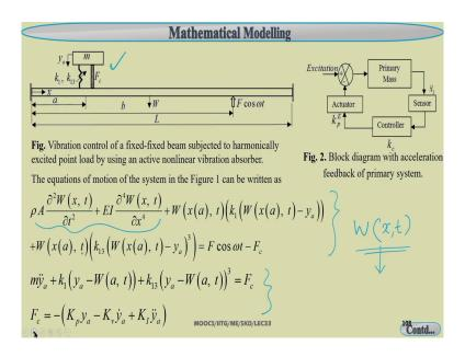
So, if you want to take so another system, I am it can show you so you can take this as a continuous system so you can in this continuous system so you can apply force F cos omega t and here this is the absorber part. So this system you can take as an assignment and you can solve the system and you can find so. In case of the beam so you can take as a different boundary conditions also. So this is a fixed beam is taken.
