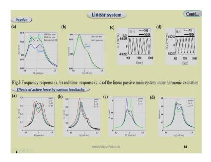
So, here also some comparison have been given these MMS 1st order MMS, 2nd order MMS and also with the one reference value. So you can see as we are using or we have a 2 degrees of freedom system, so here so one can observe 2 peaks so this is one peak and this is the other peak so these correspond to the shifting of the natural frequency or modal frequencies from the omega by omega 1 equal to 1.
