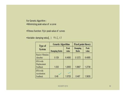
So, one can study the system there are many methods one can use; one can use the genetic algorithm also so minimizing peak value of a curve so one can use this fitness function F s peak value of the curve. So, variable damping ratio also can be taken so less than zeta a less than 1 so 0 less than zeta a less than 1. In case of genetic algorithm so some study has been carried out.
