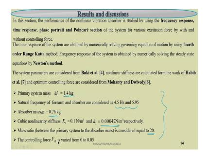
And, plotting the time response phase portrait Poincare section and using these fourth order Runge-Kutta method or by solving this set of equations by using Newton's method, one can study the system. So here, the study in the study mass is taken to be 1.4 kg, so natural frequency of forearm absorber considered to be 4.5 Hertz and 5.95 Hertz.
