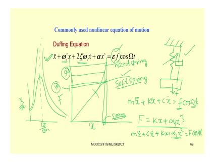
So, let us see some commonly used non-linear equation of motion. For example, let us take the duffing equation. So, in simple spring mass systems we have seen the equation of motion. So, this is a simple spring mass and damper system. So, let us put a damper also. So, in this case equation of motion is mx double dot plus Kx plus cx dot equal to if we are applying a force f then this is equal to f sin omega t or f cos omega t.
