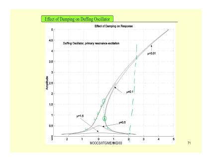
So, here at omega by omega n when omega by omega n nearly equal to 1, so, you have seen the response is maximum almost maximum and for undamped system when there is no damping so, this term this response goes to infinite. So, this is the; this is the things already you have studied.
