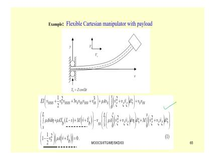
So, few more examples of non-linear equations so, you can see. So, this is a cantilever beam and here the base is excited. The system is similar to that you have seen in this previous case. So, where the platform is moving up and down and platform is excited also. In that case you can see the equation of motion. So, we will see later how the equation of motion will be there.
