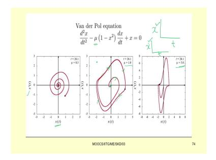
So, let us see some other ok. So, here we have plotted this thing also. So, if you plot this Van der Pol equation that is d square x by dt square minus mu into 1 minus x square dx by dt plus x equal to 0 so, you just see. So, with time you can see so, for example, taking this mu equal to 0.3.
