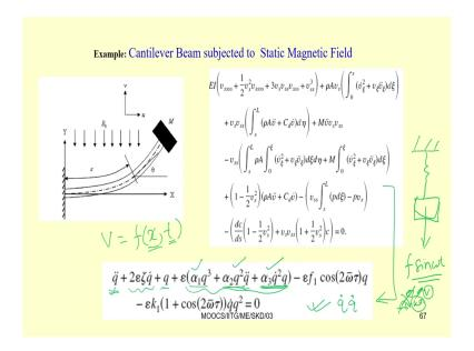
So, let us see some more examples also. So for example, same cantilever beam, so, if it is subject to a magnetic force. So, in this case you just see the magnetic force is a non contact type of force unlike your the force what I have shown for a spring mass system. So, that is; so that is the force is directly attached or force is directly applied to the system here f sin omega t force is directly applied to the system here.
