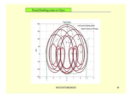
And, similarly 16 periodic you go on increasing the number of terms then you can get that this period doubling route to chaos. So, these type of curve where it is deterministic that amplitude is fixed, amplitude is bounded so, it is varying between this and this.
