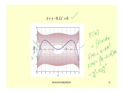
And, this instead of F u so, this will be F x. So, F x. So, these curves plots the F x versus x and if you plot the velocity versus x that is F v is nothing, but your x dot. So, if you plot x dot versus x you can get this type of curve. So, we will study more on this type of curve and what is the meaning of this curve after or in the second or third module of this course.
