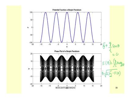
So, you can see. So, this is your F versus this theta you can put. So, for a simple pendulum this is written this curve is written for a simple pendulum. Simple pendulum equation already you know. So, the simple pendulum equation is theta double dot plus g by l sin theta equal to 0.
