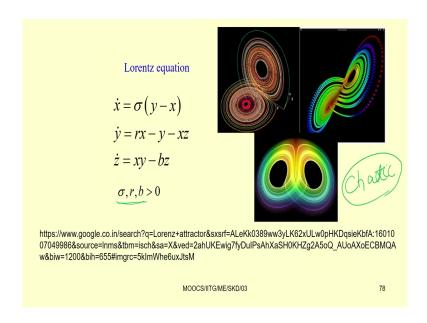
So, you may be you might have heard about another type of equations. So, here we have I have we have written three first order equation x double dot x dot equal to sigma into y minus x, y dot equal to rx minus y minus xz and z dot equal to xy minus bz. Here we have three parameters so, sigma, r, b.
