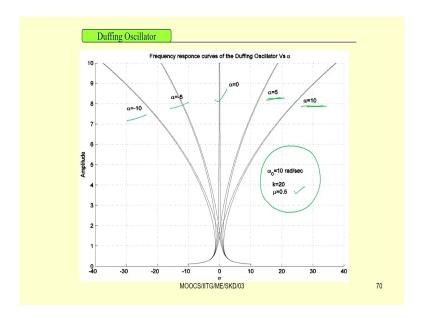
So, in this case now dividing this m in this equation so, you can write this equation in this clearly in this form that is equal to x double dot. This K by m is nothing but the square of the natural frequency that is omega n square x and then c by m can be written as 2 zeta omega n x double dot. Then this alpha 1 by m can be written as alpha x cube and then this F cos omega t F by m can be written as epsilon F.
