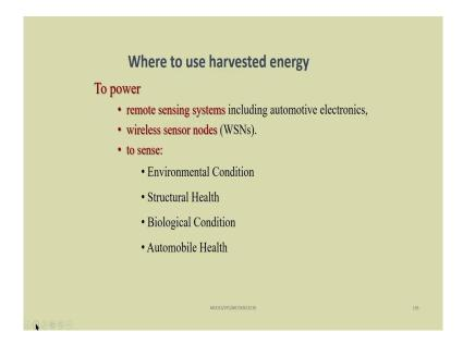
As these are the low power energy then we can particularly use them in remote sensing applications including automobile electronics wireless sensor nodes to sense environmental conditions, structural health, biological condition and automobile health and many other applications also it can be used.
