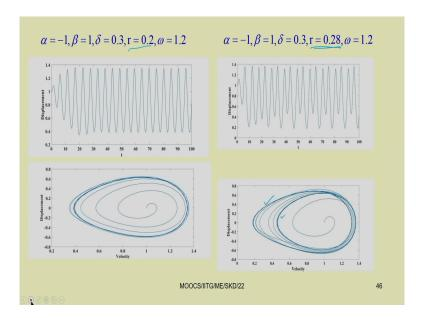
Displacement and velocity, or velocity and displacement it is up to you. So, you can plot you just see by taking this alpha equal to minus 1 that is we have taken what is alpha you just note it again. So, here in this equation, so we have taken alpha is negative, that means, the stiffness term we have taken negative.
