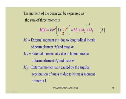
So, from this equation, so you can see the moment of the beam can be expressed as the sum of three moments these equal to M 1 plus M 2 plus M 3, where M 1 is the external moment at
