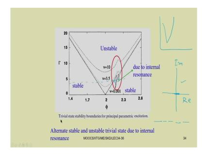
So, here you can see. So, you have plotted the parametric instability region particular a sample case has been shown here. So, for example, so in this case, so by varying these frequency and amplitude of the non-dimensional frequency and amplitude of the base excitation, so one can plot this instability region. In the previous class, we know we have used this procreate theory to plot this transition curve, also we have seen we have use this method of multiple scales also to find this thing.
