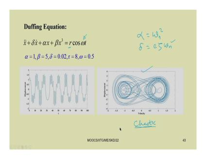
So, if we will take the duffing oscillator also, so you can observe the similar thing. So, we have written a simple code to see how the duffing equation will behave with different coefficient. So, the duffing equation can be written already you know by x double dot plus delta x dot plus alpha x plus beta x cube equal to R cos omega t.
