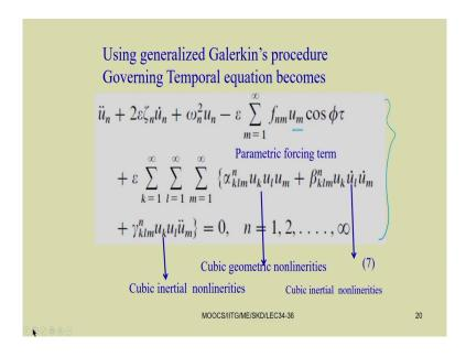
So, this way we can find this using generalized Galerkin procedure, the governing temporal equation of motions we can find. So, this is the governing temporal equation of motion. So, here you just see the equation is written in this form that is u n double dot plus 2 epsilon zeta n u n dot plus omega n square u n minus epsilon m equal to 1 to infinite f n m u m cos phi tau.
