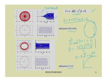
So, here you just see in case of the spring mass system. So, if we are giving some forcing term, then only it will continue to have its motion with a frequency omega. But if there is simple damping in the system, the response died out and it becomes 0. But in case of a Van der Pol oscillator, so this is the Van der Pol oscillator.
