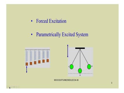
We have discussed regarding this forced excitation and also parametrically excited system. For example, in case of the forced excitations, we have a spring mass system. So, in the spring mass system, so if we have applied a force, so this is the longitudinal vibration of the spring we have seen.
