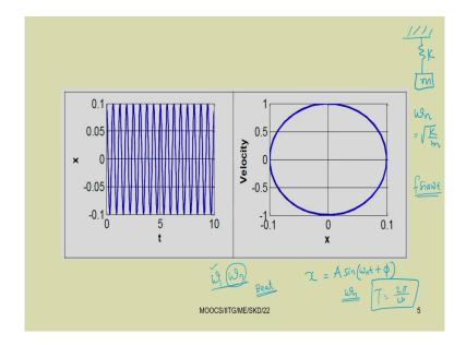
Let us start with the simple example of the spring mass damper system, spring mass system. So, if we have a simple spring and mass system, so this is simple spring and mass system. We know system will have a response so here omega n equal to root over K by m.
