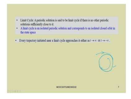
Let us see the other type of periodic response. Here we can see what we mean by this limit cycle. A periodic solution is said to be a limit cycle if there is no other periodic solution sufficiently close to it. A limit cycle is an isolated periodic solution and corresponds to an isolated closed orbit in state space. So, every trajectory initial initiated near the limit cycle approaches it either a t tends to infinite, or t tends to minus infinite.
