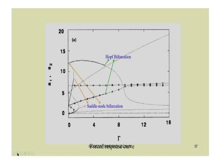
Similarly, here we can plot the force response plot. After plotting this frequency response plot, we can plot the force response plot also. So, here you just see in case of the force response, this gamma is the amplitude of the forcing. So, here you just see several type of bifurcation points.
