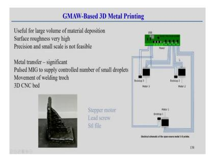
But, it is possible to develop in general, the metal printing technology using simply I am talking about the gas metal arc welding process. Here, you can see the that GMAW process is basically useful for the large volume of the material deposition, surface roughness is very high.
