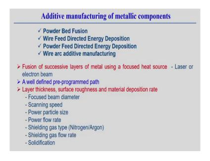
Now, if we look into in simply the additive manufacturing of the metallic component, normally there are four system can be used in general. One is the powder bed fusion powder bed fusion can be used then, wire feed directed energy deposition. Then, powder feed directed energy deposition and sometimes its a variant of these things wire feed directed energy deposition, that can be the wire arc additive manufacturing process.
