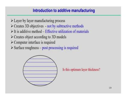
So, we can see that its simply additive manufacturing technology is simply layer by layer manufacturing process that is well known fact. And it finally, creates the 3 D objects and not by the subtractive materials rather, by depositing the material under different way it is a control way basically.
