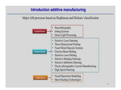
And then, the liquid has been its can be binding and the making this thing a liquid can be solidify such that the one layer can be deposited. So, liquid based the technology you can see the stereo lithography base, liquid base or its simply that some kind of the resin can be used. And the resin can be solidify using some, it can be laser or some ultra violet ray can also be used. So, that it can solidify to get the desired shape.
