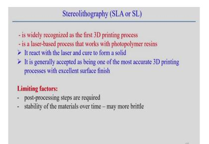
Now, we look into that process some idea about the different processes. So, we start with the stereolithography of course, the stereolithography is not exactly applicable for metallic material rather polymeric material. So, it is the widely recognized at the first 3 D printing process. And its a laser based system can be used process that works with the photopolymer resin.
