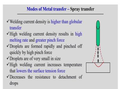
We can see from the figure also; the electrode is there, but the small small droplet can be created from the end of the electrode. And, then it can be transferred to this thing, not as a single drop transferred to the; single bigger drop transferred to the work piece metal rather than small small droplet can be created.
