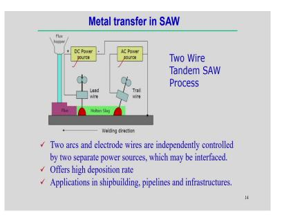
So, apart from this metal transfer and the CMT and gas metal arc welding process, we can see the metal transfer in the submerged arc welding process. But, submerged arc welding process; the we know the submerged arc welding process the everything happens this arc is over the slack or below the flux. The arc is created below the flux, this is covered with the flux arc is created and there is the metal transfer from the droplet.
