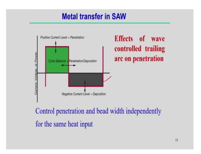
Even we can see that the metal transfer submerged arc welding process, that there is a effects of the wave control trailing arc on penetration. So, basically we can see the what we can control the penetration also in arc welding process, by simply changing this thing. So, positive current level, the current balance positive current level if it is a positive current level that actually enhance the penetration.
