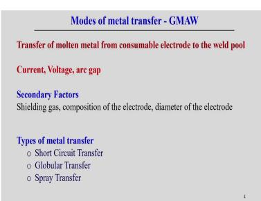
So, everything happened all the metal transfer mechanism is normally happened at the relatively low temperature, as compared to the gas metal arc welding process. Now, mode of the metal transfer in gas metal arc welding process it is basically, we understand the transfer of the molten metal from the consumable electrode to the weld pool in that is called the; there are different modes are available for the transport of the molten droplet from electrode to the weld pool.
