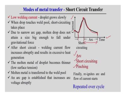
So, these are the typical condition of the spray kind of the metal transfer normally we observed, in case of the associated with the gas metal arc welding process. Now, we look into the short circuit of the another type of the metal transfer the metal transfer for circuit metal transfer. So, short circuit means, we simply understand this thing is the gap is almost 0 and
