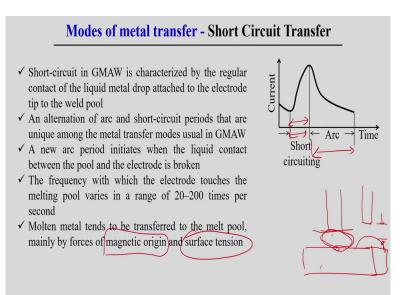
So, this phenomena actually repeated over the cycle, so this way you can explain the short circuit kind of metal transfer. Now, much more about the short circuit metal transfer we can say that short circuit in gas metal arc welding processes actually characterized by the regular contact of the liquid metal droplet attached to the work piece tip to the weld pool.
