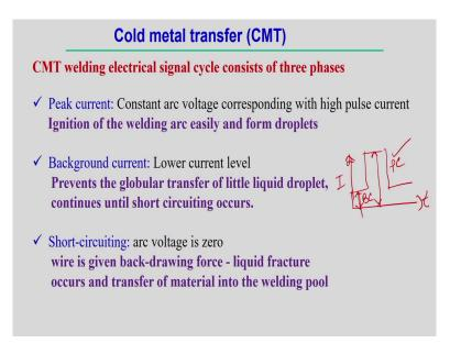
Now, in depth the CMT welding looking into this thing; how the metal transfer is as a CMT welding processes. The in CMT welding the electrical signal cycle consists of the basically the three phases. First phase is that the peak current is very important the peak current, in this case the constant arc voltage corresponding with a high pulse current.
