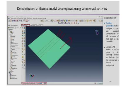
Now, selection properties, then that is assigned to a part are assigned automatically to all instances of that part in that assembly. So, basically, we can see that Abaqus colors a region green in the property module to indicate that the region has a section assignment. So, if you see region green in the this, if you see this type of marks are there.
