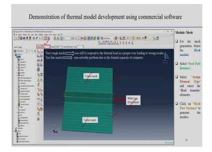
Now, this after application of the load once the load part is done then we look into the mesh that how the mesh can be done. For the mesh generation, select the mesh module. So, we see the module is the here is the module is the mesh module.
