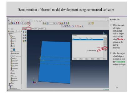
So, once it is done, then once results done, then we can see the visualization of the results. So, that means, that is also under the module job. So, under the module job, we can see that while Abaqus is solving the problem, right click on the job submitted, select the monitor to get information onto the analysis procedure.
