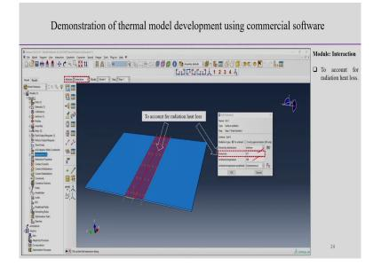
So, therefore, to account for the radiative heat loss on this particular defined zone on the surface. Then I can put the emissivity value and ambient temperature is already defined and maybe emissivity distribution, we can follow the emissivity distribution.
