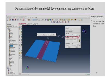
Then, we can see to account for the convection heat loss, here we can put the some value of the film coefficient, we can put the value of the film coefficient equal to 25 to account for the convective heat loss. That I can put there the film coefficient we can put this interaction.
