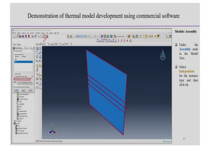
Now, this assembly module even I think till we are under assembly module, we can see the here the module assembly module. So, in this module, now we try to look into the under the assembly node in the model tree.
