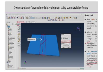
Once we do this putting click on in this particular case, we can see that we have defined this particular zone, the body heat flux is applied particular zone. So, then, body heat flux added load also we can see this particular option definition of the user defined magnitude 1 for example, user defined magnitude 1, then we can apply the that body heat flux that in the weld zone.
