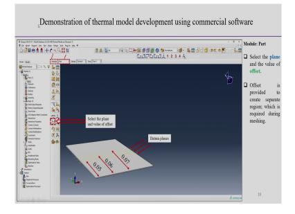
Next select the I think next till it is continue, if you remember it is highlighted, the module and the part module is basically, you are handling the part module. Now, select the plane and the value of the offset, we can put some sort of offset also. Offset is provided to create the separate zone and which is required during the meshing. So, here we can create the select the plane and the value of the offset.
