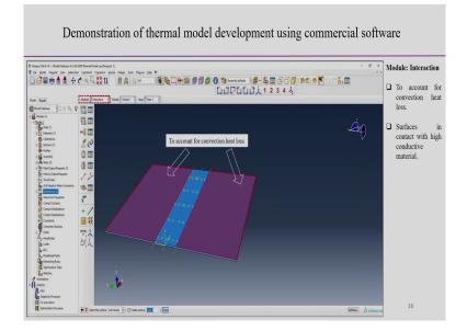
So, once we define the surface film condition, then we can go for the next step to account for the convective heat loss these two part. They are to account for the convective heat loss and the surfaces in contact with the high conductive material. So, that we can put account for the convective heat loss from this other surfaces.
