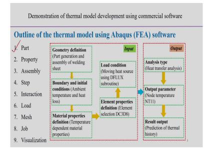
Outline of the thermal model using the Abaqus that is the finite element software we can see that there are several steps. One is if we look into that it is a; it is already I mentioned here 1 is the selection of the part or maybe defining of the part, which is or basically we can say the selection of the domain, solution domain we are supposed to calculate the temperature distribution in this particular domain.
