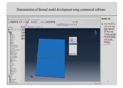
So, once it is done, then next task is the basically job. So, job is this module is the job after mesh, the module is the job. So, job in the model tree click on the job node. So, in the model tree, there you can click on the job node and from there, then click continue and then ok so, continue ok in the toolbar, click on the job manager. See here, if you see name job module 1, we continue and ok and then, we can look into the job manager also.
