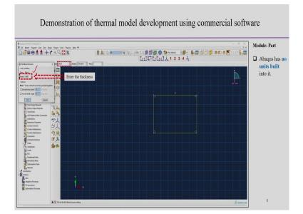
Now, enter the thickness. So, once we the rectangular shape surface we create, then we can part if you put the continue and then, we can pop with this edit the base extrusion. Here, we can see the depth we can define that we can, you can the highlighted part here we can see the depth is defined. So, here, we can see the enter the thickness here, we can put the desired thickness.
