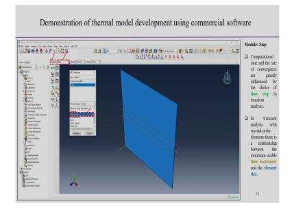
Now, here you can see. Now, we come to this next module that is the step module. The step module, the computational time and the rate of convergence definitely we know are greatly influenced by the choice of the different time step in the in this transient analysis. So, time step is very important part in the transient analysis.
