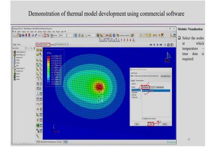
To select the nodes at which temperature time data is required for example, I can select the node for example, I want to select this particular node because the software having all the data point is the not at the particular node point. Even if you want to get the data and the in between the particular node point in the in between the node so, then it actually interpolate the data and we will be getting the results accordingly.
