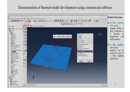
Now, this module is the interaction. So, interaction is required this module. So, module interaction how it works in this particular module interaction? Here you can see there is a in interaction 1, the surface film coefficient basically, the a film condition interaction property. Interaction property is actually defined on the surface in the terms of the film coefficient, which is as a function of temperature and field variables.
