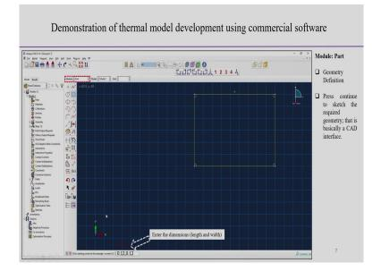
So, basically create lines means we can create the rectangle here. Now, enter the dimension, we select first the rectangle, then enter the dimension length and width. Here, we can put the enter the dimension 0.12 and 0.12 two-dimension that means, length and width we can give this thing.
