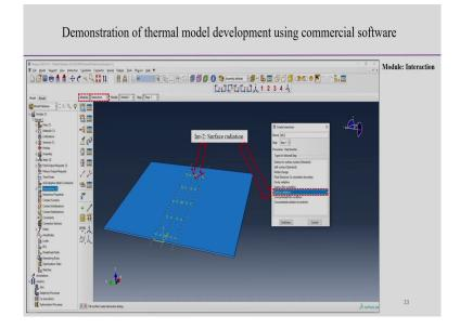
Now, surface radiation; Now, once the film coefficient defined, then you basically you are considering the convective mode of the heat loss from the surface. Now, there is a radiative heat loss also. So, in that cases, the surface radiation also has to be incorporated so, then choose the step 1, one is the then we can see the surface radiation term. So, once we choose the surface radiation term to put the properties related to surface radiation term.
