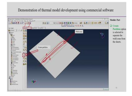
Now, create partition. So, this is the zone. Basically, this indicates the weld zone see this indicates the weld zone and this zone may be differentiate with respect to the other part. Now, create partition. So, create partition option is selected to separate the weld zone from the sheets. So, basically to separate out this weld zone so, this we define suppose we are moving
