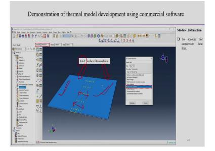
Now, surface film condition: So, surface film condition again, we come back to the surface film condition because this weld zone, this zone we have defined the film heat transfer coefficient as well as the for the radiative heat transfer, both the properties has defined already in this particular, but what should be the value in this particular zone?
