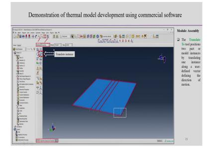
Now, translate the tool positions two part of the model instances by translating one instances along the user defined vector defining the direction of motion, ok. Now, we can put one particular direction of the motion, the translate in intense in using this particular option, we can decide the which direction heat source will be moving so, that option we have to look this thing see here, if you see.
