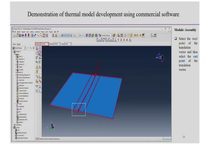
Now, assembly module, select the start point of the translation vector and then, select the end point of the translation vector. So, the heat source will be moving actually at the center point so, from here to here. So, translation motion we can put the select this point and select the end point; such that it will be automatically accommodated by the software.
