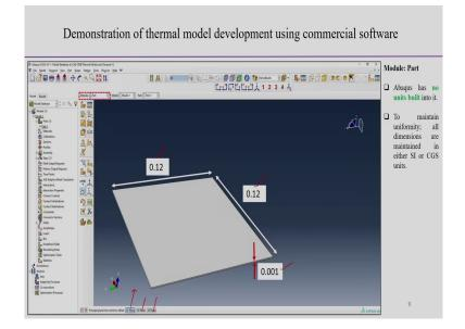
And then, we can create this Abaqus has no unit built into it to maintain the uniformity, all dimension are maintained either SI or CGS unit. So, therefore, we maintained particular unit, but it should be throughout the same unit. So, then 0.12 is the length, 12 is the width and the thickness is 0.001 so, this is the now we create the solid geometry. So, solid geometry having very small thickness in this particular case, the once the geometry has been created in this particular case.
