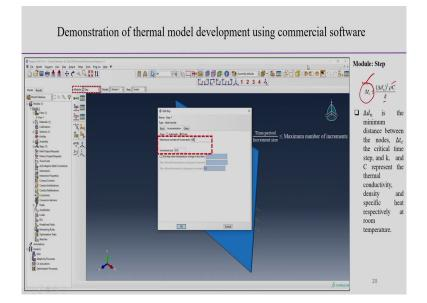
Now, see that what is the minimum time step t c is the del d n square rho C you see all the material properties are there. Del d n is the minimum distance between the nodes; between nodes. Therefore, delta times is the critical time step and k and c are represent thermal conductivity and specific heat; and the specific heat respectively and that is under the room temperature. So, then accordingly, we can decide the what may be the time step we can estimate this thing.
