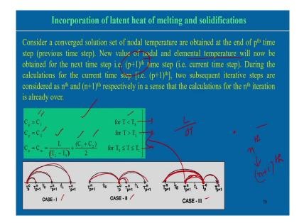
So, we can see the overall view of all this thing. Now, in a solution that set up the nodal temperature obtained at the end of the particular time step. Now, value of the nodal and elemental temperature will now be obtained for the next time step for example, p plus this thing.
