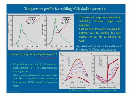
This temperature profile for welding of the dissimilar metals we can see also this a enhances the weldability the increasing temperature also. So, here you can see the temperature between aluminium, copper at the different position we can see the measure the temperature also. Without preheating figure a without preheating we can get some temperature profile, but with pre heating 55 amp we are getting this kind of the profile.
