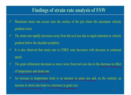
Now, findings for the strain rate analysis FSW process. So, maximum strain rate occurs definitely near to the surface of the pin are the maximum velocity gradient exist. Definitely the strain rate will be maximum near about the pin surface. Strain rate rapidly decreases away from the tool axis due to the rapid reduction velocity gradient below the shoulder.
