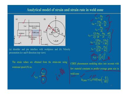
Now, it to some extent it is possible to develop in FSW process to look into the strain and strain rate this thing and to explain the recrystallization phenomena associated with FSW process also. See this cases we can see this is the tool material and the workpiece material and tool means the shoulder is interacting on the surface.
