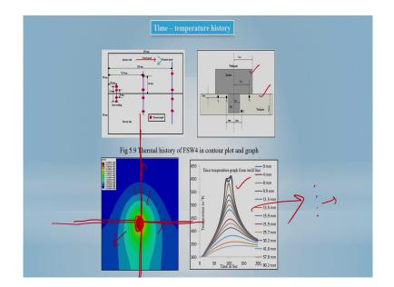
Similar time temperature history also, even we can extract the time temperature history also. For example, once you do the analysis. So, this is the interaction of the tool and the workpiece material then we can define some characteristic points. So, on this characteristic point say this is that characteristics points normally in practically we put the thermocouple on this particular point.
