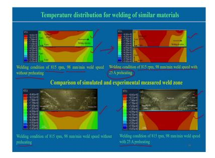
Some more results we can see the temperature distribution for welding of the similar materials. Also we can see the welding experiments for 815 rpm this is the weld speed 98 millimeter per minute and without preheating without preheating means we are not heating the sample before run of the experiment. So, we are getting some sort of temperature profile.
