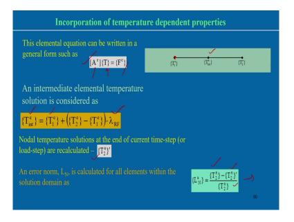
Now, incorporation of the temperature dependent properties also in the similar way can be done the other way also. For example, the elemental equation normally we finally, reach this elemental equation A T equal to F. So, that means, load and this matrix and T is the temperature. We solve this equation.
