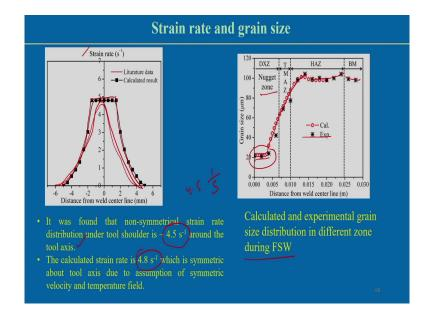
With appropriate value of all these things we can find out a distance from the a weld center we can estimate the strain rate. And this thing strain rate is that literature data, strain rate estimation is there at this particular a position. And, then calculated data a strain rate can be prediction which is close to the experimental value.
