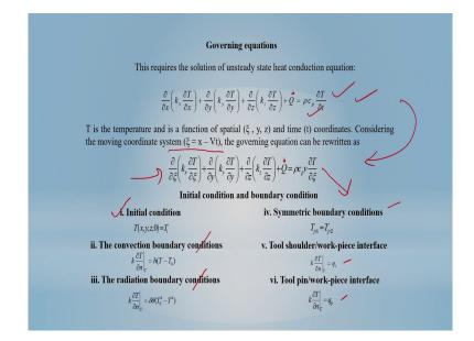
Definitely once we look into that any kind of the modeling heat transfer analysis or maybe stress analysis part. In that cases we need to know what are the governing equation. And accordingly what kind of constitute relation between stress strain, displacement strain all these kind of in relation we are using that should have some idea about all these particular processes.
