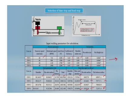
So, some sort of results we can see also welding parameters see that four different cases at the transfer speed the 40 millimeter per minute; that means, how what is the movement of the tool speed of the movement of the tool. Rotational speed rpm, tool rotational speed the different rpm 722 1400 rpm; axial force you can measure also that axial force is required during this process also.
