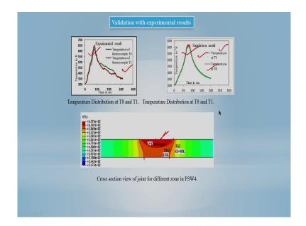
Validation with experimental results: so, here see temperature at T 1 and temperature at T 8 and temperature of thermocouple T 8 temperature of thermocouple T 1. See these are the thermocouple measure term; that means, experimentally measure temperature and this is a simulated result.
