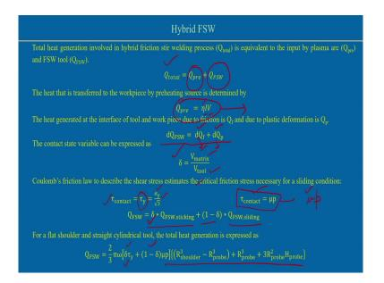
Thing is that hybrid FSW process also total heat generation involved in the hybrid FSW process is the equivalent to the heat input by plasma arc as well as the FSW tool. Now, if you look into the total heat generation in these cases the due the preheating the plasma arc and due to the FSW tool Q FSW. Now, if we look into the heat is transfer to the work piece by preheating source is determined by this way Q preheating; that means, total we know this is total heat by the arc also.
