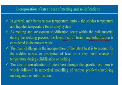
But, incorporation of the latent heat of the melting and solidification if we discuss that, normally the incorporation of the melting and solidification normally happens in the alloy system between the solidus and liquidus temperature.
