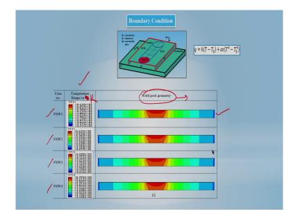
So, once you do that boundary with proper boundary condition and solving the governing equation will be able to get the temperature distribution this thing. So, it is a weld pool geometry it is not weld pool actually it is a kind of we can say the nugget zone may be you can see in FSW process.
