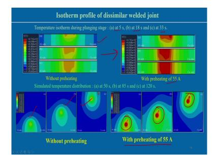
Some results also we can very get this thing without preheating the development of the temperature profile during the plunging state at the different time step 5 second, 18 second, 33 second. Here also with preheating we can get the different profile see there is difference with a preheating.
