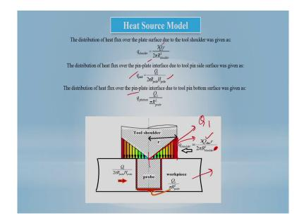
Now, once we estimate the heat generation that is a total heat generation over the surface, but maybe we do not have the actual implement in this model you have to incorporate the in the form of a heat flux on the surface. Here you can estimate what is the total heat generation now on this particular surface or at the contact surface.
