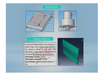
Therefore, you can create some sort of suppose this is a model geometry at sample geometry we can create. Then this is the tool dimension if we defined, this is the shoulder on the shoulder. And this is the tool pin and accordingly the analysis the work piece is meshed using the brick element.
