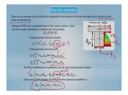
So, let us look in the how what way we can do the heat flux calculation in FSW process in. So, this case there are two process due to which the heat is generated at the interface, one is the interface means if you see this is the tool and then at this one heat generation will be at this a interface between the shoulder and the workpiece.
