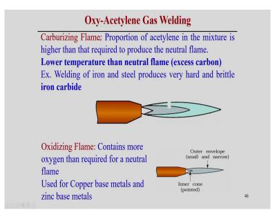
Apart from the neutral flame carburizing flame can also be created, but in this case definitely acetylene ratio of acetylene percentage will be more in this case. So, proportion of the acetylene in the mixer is higher than that of the required to produce the neutral flame. So, in this cases lower temperature than neutral flame because of the formation of the excess carbon.
