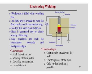
Similarly, electro slag welding process in this case the workpiece is filled with a welding flux. These two workpiece are there in between the gap is filled with the welding flux. Then at start, arc is created to the melt the flux powder and the forms molten slag.
