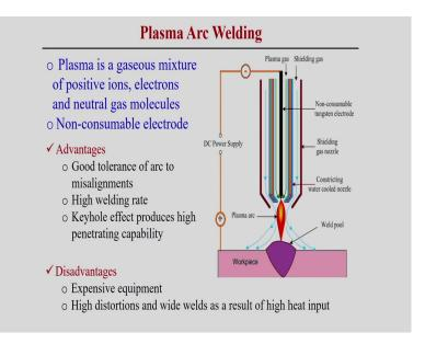
Now, if you can look in to the plasma arc welding plasma is a mixture of the positive ions electrons and neutral gas molecules, but in this cases the plasma arc welding process which is different from the gas metal arc welding process. In this case there is a two source of the gas is required.
