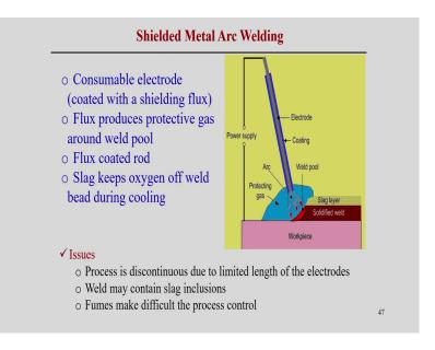
Now, we will look into the different other welding processes. The shielded metal arc welding process shielded metal arc welding process we can see that we can use the consumable electrode and coated with a shielding flux. So, electrode is coated with the flux from this figure and arc is created.
