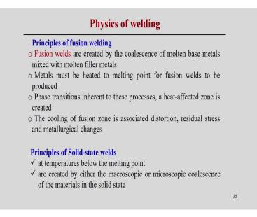
Now, principle of the fusion welding process we can see that fusion welding means their application of the heat such that it creates at least reach the melting point temperature and the coalescences by these two component base metals and sometimes mixed with the filler materials, but it is not necessary you have to use the filler materials autogenous fusion welding is also possible.
