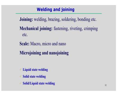
Now, we start with this thing welding and joining. If we look into that over all we can always say that it is a kind of welding and joining processes not only welding or not only joining processes because in some part you can categorize these joining processes something like that it is includes all these processes welding, brazing, soldering, even bonding.
