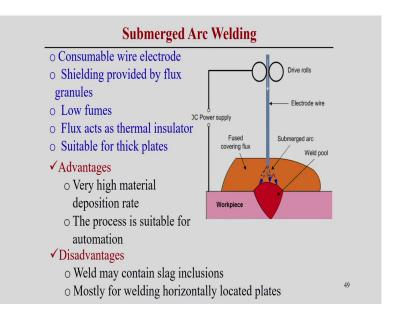
Now, submerged arc welding process: submerged arc welding process also use a similar kind of different from the gas metal arc welding process. Here also electrode wire is used, but instead of shielding gas it is used the fused covering flux, the total weld zone is covered with the fused covering flux and arc is created under the flux and weld pool is created. But, how it is different from the other process?
