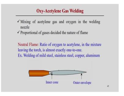
Now, I come to the different welding processes we can start that oxy acetylene gas welding process. Now, I come to this point the different fusion welding process one is the oxy acetylene gas welding process simply mixing of the acetylene gas and oxygen in particular ratio in the wielding purposes.
