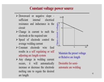
One is the constant voltage power source. In this case constant voltage is maintain the preset voltage or relative arc length. Basically the in arc welding process the arc voltage is very much relevant to the voltage is basically set relevant to the arc length. So, it is very much sensitive to the arc length.
