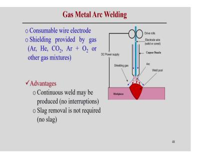
But, I will look into the gas metal arc welding process use the similar principle, but in this case there is a continuous supply of the wire is required. So, consumable wire electrode: so, from the pool of the wire there is a continuous supply of the wire is there.
