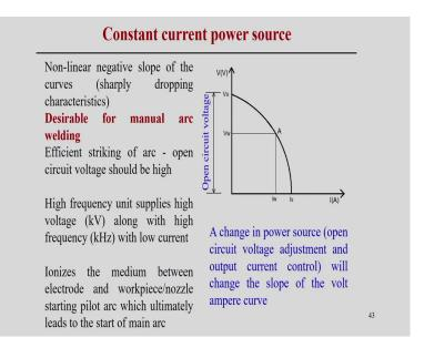
Now, other look if the if you see the that is called the sharply constant current or falling characteristic of the power source. You can see the figure indicates the open circuit voltage, but there is a sharply dropping characteristic of the current is there. So, non-liner negative slope of the curve sharply dropping characteristics normally follow in case of constant current power source in this case desirable for the manual arc welding process.
