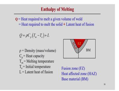
Now, enthalpy of melting because it is necessary to understand what we can say the what is the enthalpy of melting; that means, basically heat content in a particular welding process what we can estimate that may be helpful for the development of the model and that we will see also later on, but here we can see the enthalpy of melting heat required to melt a given volume of the weld.
