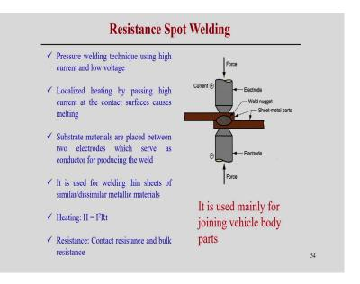
Now, we can also look the resistance spot welding process that is another welding processes where pressure of the electrode is required using the high current and low voltage. So, this is the principal of the resistance spot welding process.
