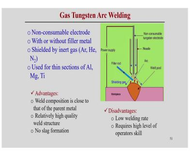
Now, gas Tungsten's arc welding process. In these cases we use the non consumable electrode and sometimes if necessary we can use the some filler rod externally. Same principle non-consumable electrode; so, if a current is pass electrical circuit is if you can see between the electrode and the workpiece and the weld pool has been created, arc has been
