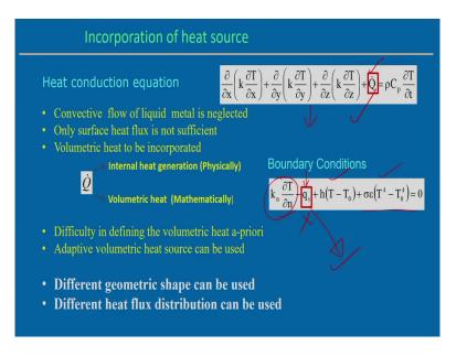
So, first start with this different heat sources model, but what way we can incorporate this heat flux or distribution of the heat flux heat intensity into the model into the heat transfer model. So, this heat conduction equation we know this is the 3 dimensional heat conduction equation, we use that this term the highlighted part is that Q dot that is called the.
