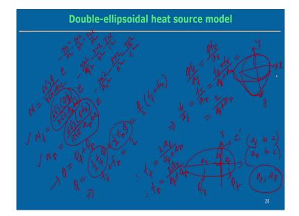
Now we can see what we can estimate the double ellipsoidal heat model. So, a ellipsoidal heat source model how what we can be extend to double ellipsoidal heat source model. So, now, that we see that we use some ellipso having the axis line a, b and c, but in case of ellipsoidal model is more suitable in case of the stationary heat source model, but suppose there is a heat source is moving on particular direction for example, this is the x axis and this is y axis and z axis.
