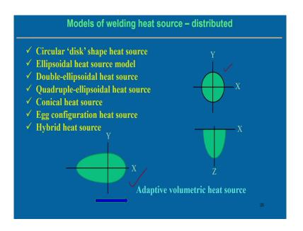
Hello everybody today we will discuss the models of the welding heat source, last class we have discussed the analytical solution of the different heat source are associated with the welding process, but in analytical solution we assume that heat source can be represented like a point heat source kind of line heat source and based on that with other assumptions.
