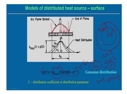
So, models of the distributed heat flux on the surface and we can see that what we can incorporate this thing. Just let us look into the surface heat flux only. So, this figure indicates that this is the typical arc the shape of the arc. If you look into the what are the typical shape of the arc that the intensity and the gap is there is the arc at the intensity this is the maximum and the intensity is gradually decreasing both the sides in this form, this is the typical shape of arc.
