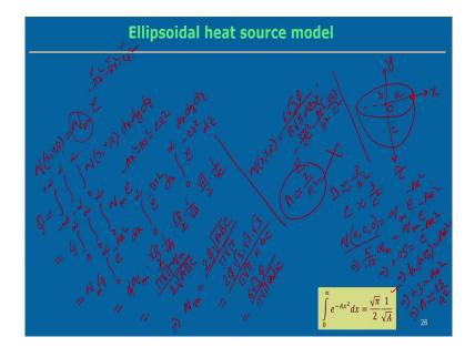
So, ellipsoidal heat source model we can see that in case of the ellipsoidal heat source model that we normally using gives the spot welding process we can see an ellipse kind of this thing as being that these are the 3 different axis. So, semi major axis a y axis b and z it is the length semi axis length equal to c.
