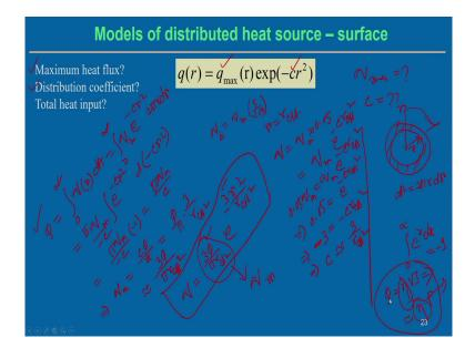
So, that we have to look that what we can estimate the heat flux density distribution. So, in this case we can see that q r can be represented to the q max are exponential seen to r. So, these two things are there what is the maximum value of the heat flux. So, what is the value of q max that has to be estimated and what is the distribution coefficients value that has to be estimated we can estimate this thing and this curve.
