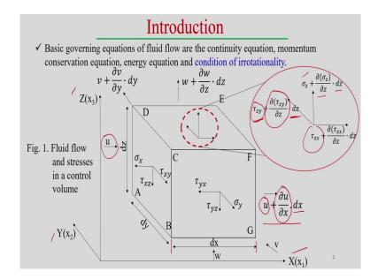
So, to start with this first we will look into how basic governing equation of the fluid flow are in the normally develop. So, there is a if you see look into this basic aspects associated with the fluid flow also is the first is the continuity equation, momentum equation even also energy conservation equation as well as the condition per irrotationality.
