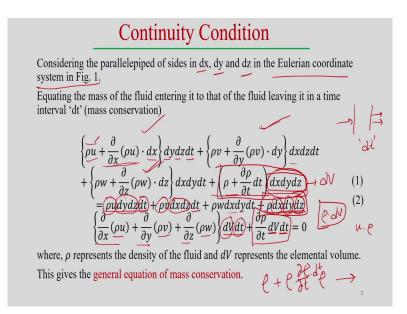
So, let us considering the parallelepiped of the sides of the dx, dy and dz that way. The Eulerian coordinate system I already explained in the figure one. Now, equating the mass of the fluid entering to that of the fluid and which is entering to it and that of the fluid living it at time interval dt.
