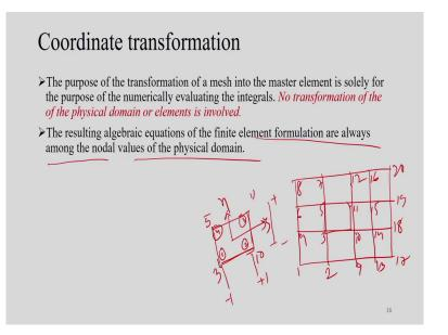
Now, coordinate transformation is something like that. The purpose of the transformation of the mesh into a master element is the solely for the purpose of the numerically evaluating the integral. So, that is that will be easier. So, all the coordinate transformation is required in this case.
