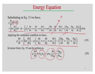
So, now if we substitute all this expression in incremental we have the this thing rho del e by del t into dV into dt. So, that we can see also and that is the; that is the expression 13 we can we are considering from there. This is the incremental strain energy and this is the energy in and out balance and that means, from there.
