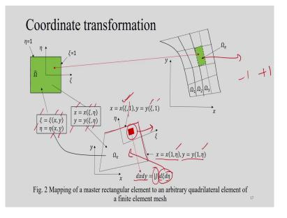
You can see the also coordinate transformation the similar way the mathematically we can express like this suppose this is the; this is the actual domain one particular domain pick up this domain. We can transport this thing local coordinate system coordinate transformation here we can see the this thing.
