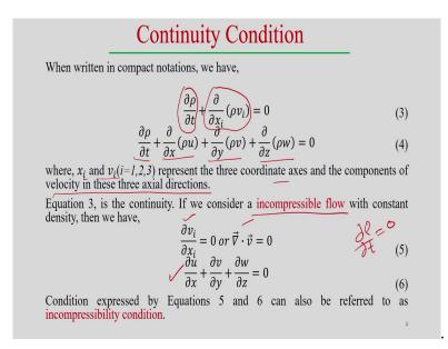
And, then we are getting in the compact from the notation we can find out the del by del rho by del t and this del by del x i equal to v i, the i equal to 1, 2, 3. So, that means, x 1, x 2, x 3 or x, y, z. Now, expand this one also other way also in terms of x, y, z. So, the x component del by rho dz and del rho by del t equal to 0; so, that comes from the elemental volume.
