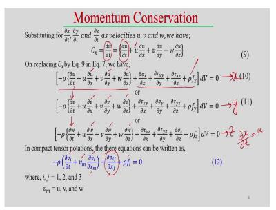
So, now substitute d del x by del t. So, similarly in that case is del x by del t we can see this also velocity along the x-axis this is can be represented like the u velocity component. So, similarly del y by del t, del z by del t all the velocity components; so, u v and w along the x, y and z direction. So, from there we can find out what is available C x.
