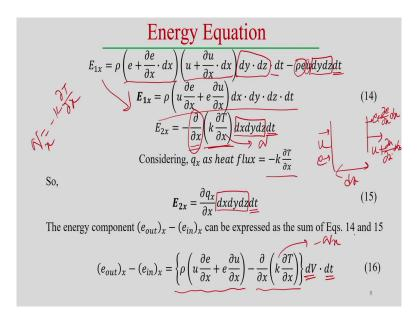
So, rho e into change of the energy with respect to because over the spatial domain dx even this thing and at the same time there is a change of the velocity also, the spatial domain one is the exit. So, here is the velocity was u and there is a one entry level and exit from this
