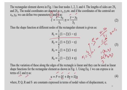
Now, we will see what we can map from global to the local coordinate system. Now, the rectangular elements shown in this figure has the four nodes 1, 2, 3, 4 the length of the sides
