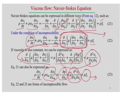
And, in that case what is the Navier-Stokes equation we can find out. We can this Navier-Stokes equation actually can be expressed in a different way from the equation number 12, such that we can get the velocity component and the this velocity components also there and the pressure is also comes into the picture.
