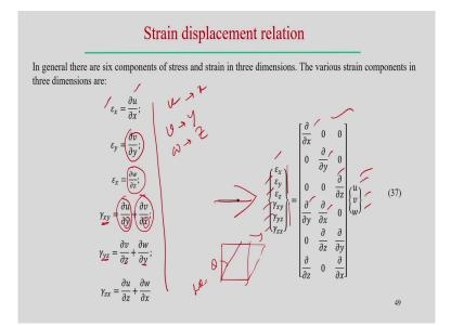
Now, look into the other aspect here you can see the relation with the general expression for the six components of the stress and strain in the three dimensional form. So, therefore, we know that strain the small strain, but in the small deformation is there; then strain epsilon x along the x axis this can be relate the between the displacement field and the strain is something like that del u by del x. But you remember use the variable, is the displacement along x axis.
