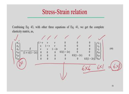
Now, combining this expression in terms of the shear stress and shears all the stress components, this stress components sigma x, sigma y, sigma z, tau x y, y z and z x all the stress components are there. And in this particular case, we write in this in the matrix form and this is the strain component; all the strain components are there.
