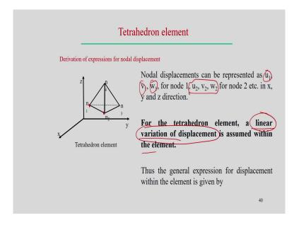
So, we can consider the, even not exactly not necessary always we have to consider the brick element, rather we can consider only on the tetrahedron elements; and that tetrahedron elements is the whole domain; we divide, we mess, put the mess in such a way that it will create only on the tetrahedron element.
