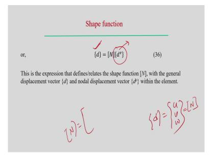
So, once we get this thing, but general expression we can see d; displacement filed the d is basically indicates the displacement field u, v and w. And this can be represented the shape function N and d e; d is the basically the nodal displacement, we can see the displacement is defined each and every of the node point for this particular element. So, this is the expression for the defines, relates the shape function N, with the general displacement vector d and the nodal displacement vector.
