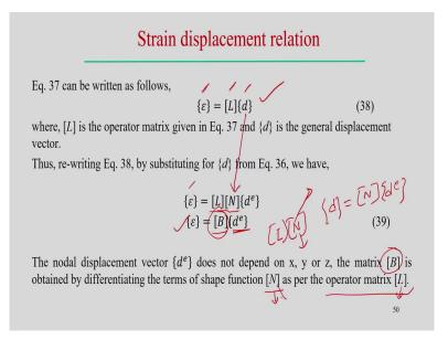
So, these are the expression the strain versus displacement field. Now, more general way we can see that this that can be written in the previous equation can be written e epsilon is the in general strain field variable and L is the operator matrix and d is the. So, general displacement vector, L is the operator matrix and epsilon is the strain field.
