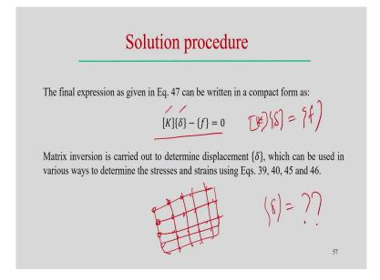
Now, general expression is that, if you look into the dimension of this matrix or column vector, all this can be represented in general way that, K delta equal to the stiffness matrix, delta is the displacement field and f counts all the this thing; f counts all the basically the load acting on the solution domain.
