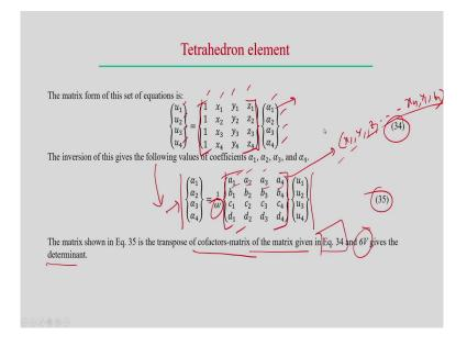
So, therefore, in the matrix form, we can write this equation like that. So, in this case we can see the u 1, u 2, u 3, and u 4; but it should be like that, it is a third bracket. And here the matrix form we write that, put according position alpha 1, alpha 2, alpha 3, alpha 4; this is simply representation of the 4 linear system of the equation in the form of a matrix.
