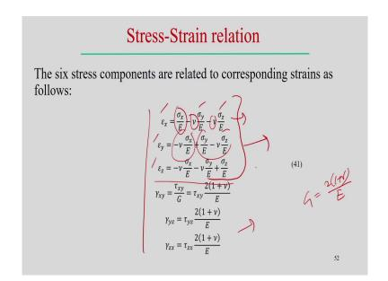
Now, stress strain relation, we have already seen that the; we have already seen that how the displacement and strain field can be related. Now, similar way the stress versus strain can be related and we have already shown that, how the, what is the in case of if we look into the elastic up to the elastic, within the elastic limit, what way the stress and strain can be relate. Those strain can be relate in this five six component of the strain epsilon x, epsilon y and epsilon z.
