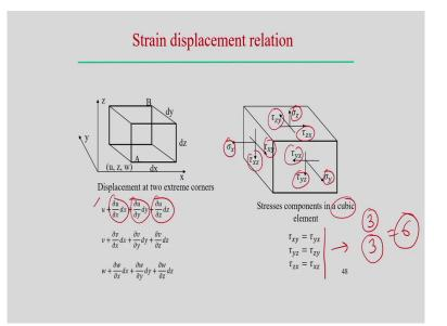
Now, strain displacement relation. We have already seen the strain displacement relation in case of, then two dimensional element, how we can relate between the strain and displacement; because this is also necessary. And we have already explained this thing when you are looking into the strain displacement relation; we are assuming the small deformation theory.
