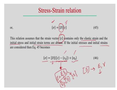
Now, stress strain finally relate the stress equal to, this is the strain and D. D is basically takes care of all this accounting the D is basically associated with the material properties. So, basically Young's modulus and the Poisson's ratio and different expression of this D matrix the form, shape of the D matrix will be different in case of two dimensional or in case of the three dimensional.
