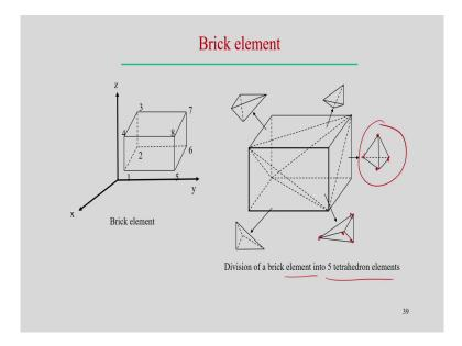
So, let us start with the brick element. If we look into this brick element and we put when you look into one brick element; one particular element for a whole domain we consider and this is normally called the brick element. And you see the numbering is 1, 2, 3, 4; there are 8 node points associated with this brick element and we define in such a way that, we have already explained this thing, numbering can be done in such a way that it should follow some particular sequence.
