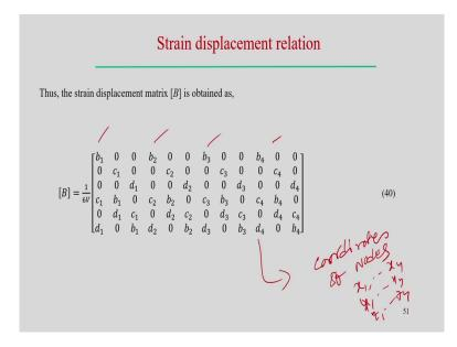
So, therefore, the strain displacement matrix B can be obtained as like that; so now, if we look into that, previous thus for linear element. So, in this case is the linear element in the sense, the displacement vary linearly within this element. So, in that case, the shape function if we remember the; it is a linear function of x, y and z and L is the operator matrix.
