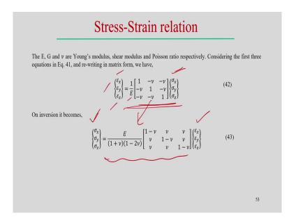
So, we can see that E, G and nu are the Young's modulus, shear modulus, Poisson's ratio respectively. So, considering the first three equation of the equation 41; that means if we look into only the normal strain component, then first three equation if we consider, then we can relate between the strain versus stress is the in terms of the Young's modulus in the matrix form.
