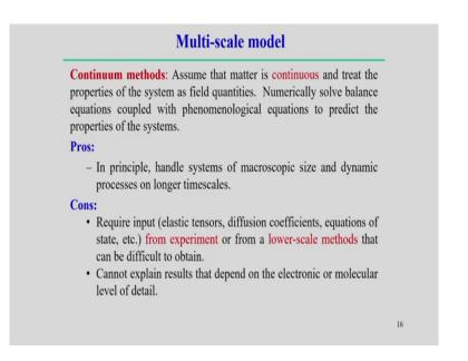
Continuum methods therefore, this method is assume that the matter is continuous and this treat the properties of the system as a field quantities. Numerically solve the balance equations coupled with the phenomenological equations to predict the properties of a particular system.
