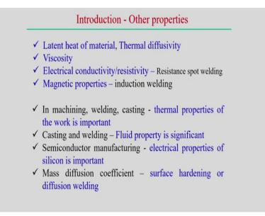
Other properties also in associated with the modelling approaches for example, latent heat of material. So, it is associated with the phase change from liquid phase to solid phase or vice versa. So, from solid phase to liquid phase or latent heat of solidification, both are important that can also be measured.
