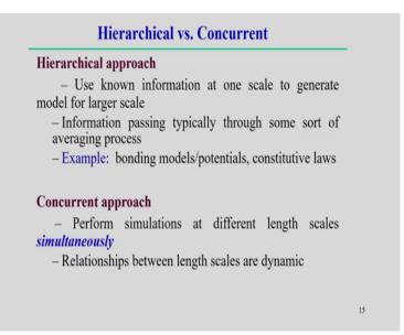
Now, it just definition which on the hierarchical approach and concurrent approaches. So, hierarchical approach use the known information at one scale and to generate the model for the larger scale. Basically we get the information in the lower scale and the supply this information to the larger scale to develop that model.
