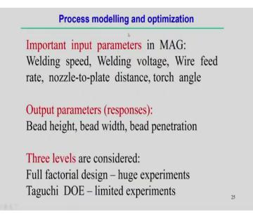
Now, input parameters can be in a MAG welding process and for example, welding speed, welding voltage, wire feed rate nozzle to plate distance torch angle. This can be done and the output parameters at the different responses for example, a height bead width bead penetration these are the output parameters.
