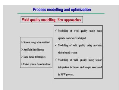
We take one example pertaining to the welding process. The what are the few approaches. So, sensor integration method; that means, it is a collection of the data and analysis of the data method. We can use any artificial intelligent techniques also. We can use several data based techniques; that means, some statistical methods we can use it.
