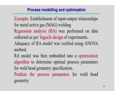
Now, it will be more easier to understand that what we can do the process modelling and optimization these things ah. We can take an example of the MAG metal active gas welding process and here what we can establish between the input and output relationship. We can simply the regression analysis which is collect the data and as per Taguchi design of the
