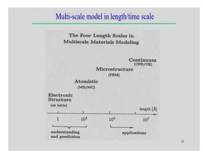
That is why multi-scale model at the different length and time scale can be divide in broadly in this four categories the four length scale in the multiscale materials modelling. Here you can see that starting from the electronic structure. Electronic structure basically exists in this thing at the very lower scale in the may be nanometer or less than nanometer scale.
