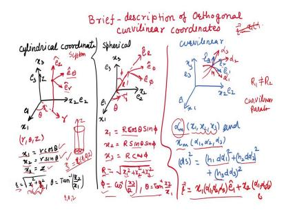
Today we will discuss the Strain Displacement Relations and representing the strain displacement in a curvilinear coordinate system. I will explain briefly about the orthogonal curvilinear coordinate system. The very first system all of you aware of is the cylindrical coordinate system.
