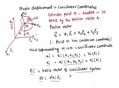
The basic steps to derive a strain displacement relation in the curvilinear coordinate system is let us say point M, located in the 3- D space having position vector r and the curvilinear parameters  $\alpha_1$ ,  $\alpha_2$ ,  $\alpha_3$  and this position vector  $r = x_1 \overline{e_1} + x_2 \overline{e_2} + x_3 \overline{e_3}$  then,
