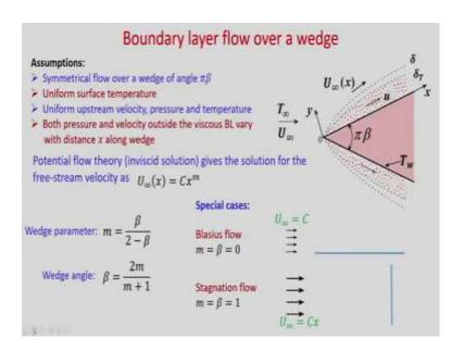
So, let us consider laminar boundary layer flow over a wedge. This is the case. So, you can see this is the wedge, with the wedge angle  $\pi$   $\beta$  and your free stream temperature is  $T_{\infty}$  and free stream velocity is  $U_{\infty}$ , x is measured along the surface and y is normal to the surface. So, obviously, you can see when fluid will flow over this wedge, it will be accelerating; the fluid velocity will accelerate.
