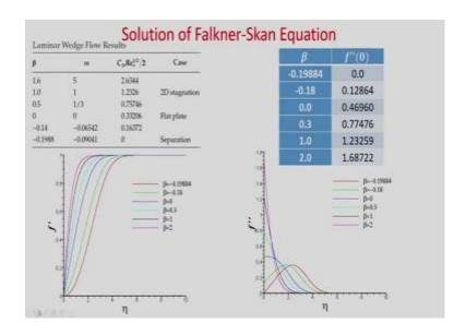
So, if you see laminar wedge flow, so for different  $\beta$  and corresponding m value is shown here and if you see  $C_{fx} \frac{\text{Re}_x^{1/2}}{2}$ , this value if you see here then, you can see for  $\beta$ =0, m = 0. So, what is your f "(0)? That means, your velocity gradient at the wall. So, that is 0.33206. So, that you have already found, right. So, this is the flat plate case.
