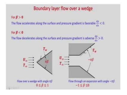
So, here you can see two different situations for  $\beta > 0$ . So, in this case you can consider that, flow over a wedge with angle  $\pi$   $\beta$  and  $\beta$  varies between 0 and 1, then the flow accelerates along the surface and pressure gradient is favourable. Because  $\frac{dp}{dx} < 0$ , so pressure gradient will be favourable and flow will accelerate.
