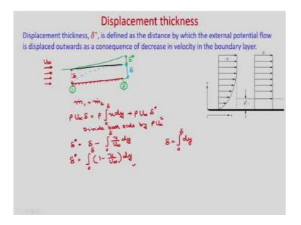
Now, let us define displacement thickness, momentum thickness and shape factor for boundary layer flow. So, first let us discuss displacement thickness. Consider just free stream velocity  $U_{\infty}$ . So, if you consider this case then obviously, you can see your stream line will be all parallel to each other, right.
