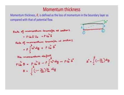
Now, we will talk about the momentum thickness. So, momentum thickness  $\theta$  is defined as the loss of momentum in the boundary layer as compared with that of potential flow.
