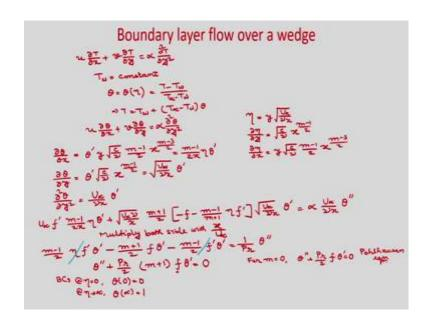
So, if you see we have written the energy equation as  $u\frac{\partial T}{\partial x} + v\frac{\partial T}{\partial y} = \alpha\frac{\partial^2 u}{\partial y^2}$ . So, now, already we have the transformation details. Here, we are assuming  $T_w = \text{constant}$ . And, we are assuming  $\theta$  is function of  $\eta$  only,  $\theta = \theta(\eta) = \frac{T - T_w}{T_w - T_w}$ . So, from here you can see,  $T = T_w + (T_w - T_w)\theta$ .
