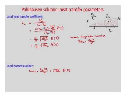
So, local heat transfer coefficient  $h_x = \frac{q_w^*}{T_w - T_\infty}$  and this we are writing from the Newtons
