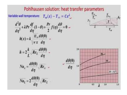
So, you can see variable wall temperature  $T_w(x) - T_\infty = Cx^\lambda$ , and this is the Pohlhausen equation right. So, this is the ordinary differential equation. So, for a special case we put  $\lambda = 0$ , where wall temperature become constant; so we drop this term.
