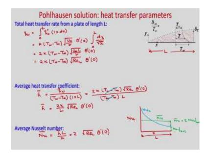
Now, let us calculate the total heat transfer from the plate of length L and we will calculate it for unit width. So, total heat transfer rate from a plate of length L you can calculate  $q_w$ . So, just local heat flux you have calculated into area. So, per unit width so, it will be,  $q_w = \int_0^L q_w^* (1 dx)$ . L is the length of the plate.
