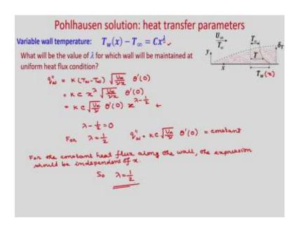
So, this is your variable wall temperature  $T_w$  is function of x. Now, what will be the value of  $\lambda$ , for which wall will be maintained at uniform heat flux condition? So, we have
