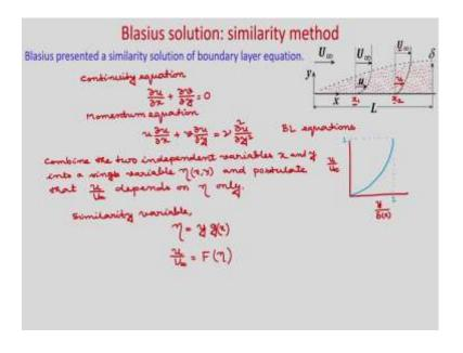
Now, let us consider flow over flat plate. So, this is the simplest solution we can do for flow over flat plate, because your pressure gradient is 0. So, first let us write the governing equation. We have already derived the boundary layer equations for flow over flat plate. So, continuity equation; so, what is continuity equation?  $\frac{\partial u}{\partial x} + \frac{\partial v}{\partial y} = 0$ .
