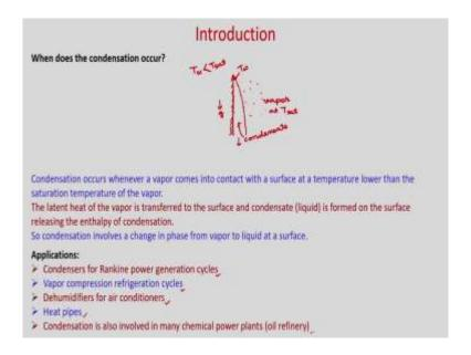
We can ask this question, when does the condensation occur? So, when the vapor comes into contact with a liquid or a surface which has less temperature than the saturated saturation temperature of that vapor, then condensation will occur. When the vapor comes into contact with a cold liquid then condensation may occur and it may form fog.
