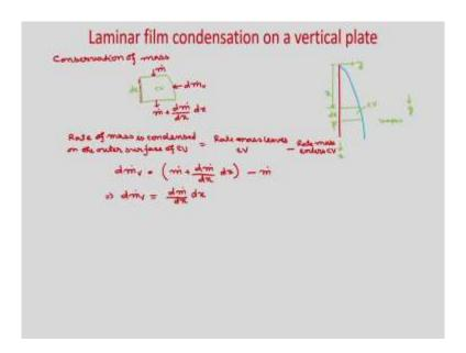
So, if you consider the vertical plate and this is your film thickness, this is your y, this is your x, g is acting in downward direction and if you consider these elemental volume where you can see if it is vapor. So, from the vapor it will release the latent heat through this interface and this will conduct to the surface and in the surface it will release the heat.
