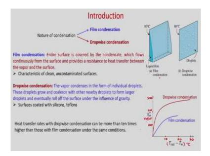
So, you can see film condensation generally one film is formed on the surface and this film just come in downward direction due to gravity. So, this is known as film condensation. So, entire surface is covered by the condensate which flows continuously from the surface and provides a resistant to heat transfer between the vapor and the surface.
