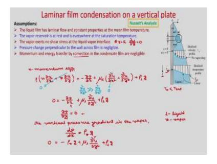
So, these are the assumptions are made. The liquid film has laminar flow. It is steady laminar flow and constant properties at the mean film temperature. The vapor reservoir is at rest and is everywhere at the saturation temperature. The vapor exerts no shear stress at the liquid vapor interface; that means, if you have, this is the vertical plate.
