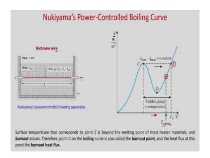
So, you can see it was his experimental setup. This is a power control heating. So, you have this voltage difference and the current is passing through this nichrome wire. And he was just increasing the heat flux on this nichrome wire by controlling the current.
