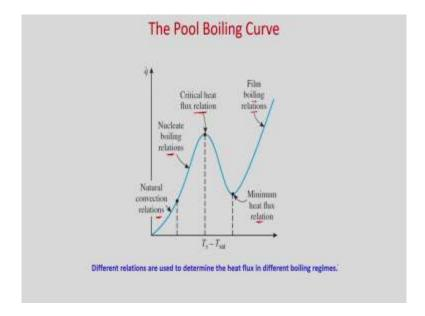
So, we can see we have natural convection relations where your natural convection takes place, then nucleate boiling relations, then critical heat flux relation where maximum heat transfer will take place, then minimum heat flux relation at the Leidenfrost point whatever heat flux you get, then film boiling relations. So, different relations are used to determine the heat flux in different boiling regimes using correlations.
