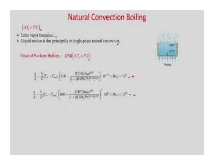
So, you can see this natural convection boiling takes place when your excess temperature is less than 5  $^{0}$ C. So, there will be little vapor formation liquid motion is due to principally due to single phase liquid motion is due principally to single phase natural convection. And onset of boiling takes place at 5  $^{0}$ C.
