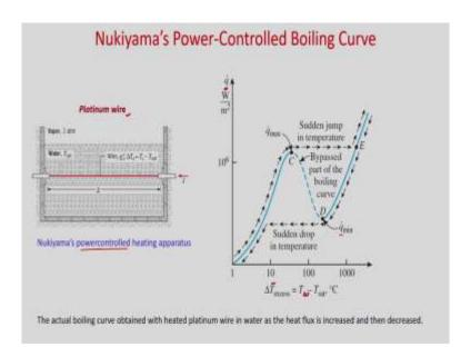
So, when he used platinum wire in the same experimental setup and he was controlling the power, that means, he was increasing the heat flux then he observed that you can see here. So, when he was increasing the temperature, it was following this natural convection regime, nucleate boiling regime.
