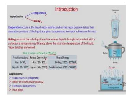
So, first we will discuss about the vaporization. Vaporization is a phase change process where phase change occurs from liquid to vapor. So, vaporization can be classified as evaporation and boiling. Evaporation is a surface phenomena and boiling is a bulk phenomena.
