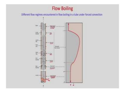
So, water, subcooled water is entering here. Now, the surface of the tube is maintained at constant wall heat flux. So, when this liquid flows through this tube, there are different regimes are seen. You can see that when subcooled liquid enters here, so obviously, the there will be forced convection because the temperature of the liquid will get heated. Once you go up, then you will see that there will be subcooled flow boiling will takes place.
