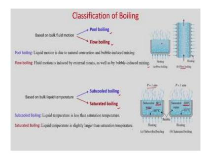
Let us discuss about the classification of boiling. So, we can see based on bulk fluid motion, you can classified classify as boiling can be classified as pool boiling and flow boiling. In case of pool boiling, your liquid medium is quiescent. Once the heating starts, so there will be natural convection.
