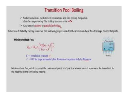
Now, if you go beyond that regime, then you will get transition pool boiling. So, in a transition boiling, what happens it shifts between nucleate boiling and film boiling. So, surface condition oscillates between nucleate and film boiling, but portion of surface experiencing film boiling increases with your  $\Delta T_e$ , also termed unstable or partial film boiling.
