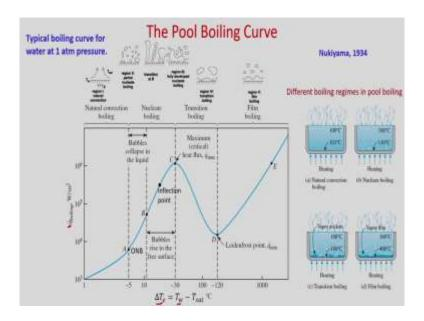
So, when you use temperature controlled curve, so that means, your controlling  $\Delta T_e$ , that means,  $T_w$  you are increasing slowly and you are measuring the heat flux. In a, what Nukiyama did Nukiyama, initially he was actually maintaining the heat flux. So, he was increasing the current. So, heat flux was increasing and we discuss about the boiling curve.
