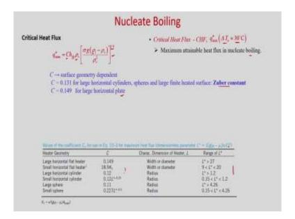
So, as a temperature increases, you can see surface tension decreases. Then at the in the nucleate boiling, you will get the critical heat flux. So, this critical heat flux you will get when your excess temperature is of the order of 30  $^{0}$ C. So, this is the maximum attainable heat flux in nucleate boiling.
