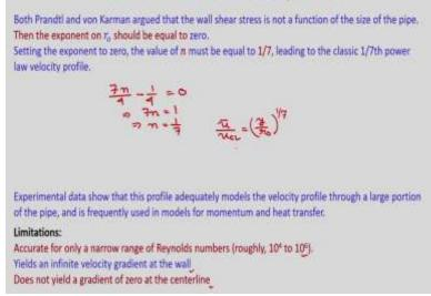
Now, we need to find the value of exponent n both Prandtl and von Karman argued that the wall shear stress is not a function of the size of the pipe then the exponent on  $r_0 = 0$ .
