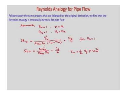
Now, first let us discuss about the Reynolds analogy because we have already derived for laminar flows and for a special case when Pr = 1 and turbulent  $Pr_t = 1$ ; that means, your kinetic viscosity is equal to turbulent viscosity and also your thermal diffusivity is equal to your eddy diffusivity.
