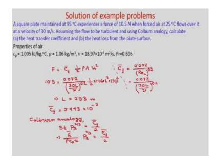
Now, let us solve two problems. A square plate maintained at 95  $^{0}$ C experiences a force of 10.5 N when forced air at 25  $^{0}$ C flows over it at a velocity of 30 m/s. Assuming the flow to be turbulent and using Colburn analogy, calculate (a) the heat transfer coefficient and (b) the heat loss from the plate surface.
