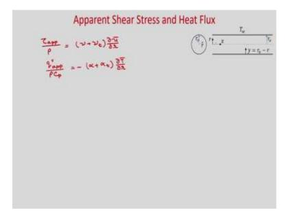
Now, whatever we have derived the apparent stress and apparent heat flux flow over flat plate those will be applicable for pipe flow. So, you can write  $\frac{\tau_{app}}{\rho} = (v + v_t) \frac{\partial u}{\partial r}$  and
