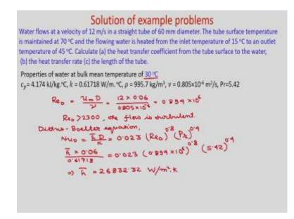
Now, let us discuss about the next problem. Water flows at a velocity of 12 m/ in a straight tube of 60 mm diameter. The tube surface temperature is maintained at 70  $^{0}$ C and the flowing water is heated from the inlet temperature of 15  $^{0}$ C to an outlet temperature of 45  $^{0}$ C.
