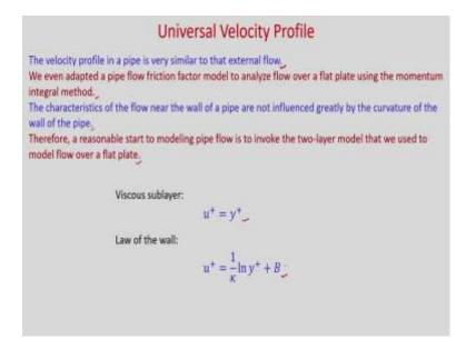
For flow over flat plate case already we have derived the universal velocity profile, we considered very small region near to the wall and we assumed that their shear stress remain constant. So, that is your viscous sub-layer and away from the wall you have law of the wall. So, the velocity profile in a pipe is very similar to the external flow.
