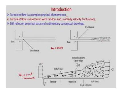
Generally turbulent flow occurs relatively at high Reynolds number and in turbulent flows velocity temperature fluctuate with time. Turbulent flow is a complex physical phenomena, turbulent flow is disordered with random and unsteady velocity fluctuations. In laminar flows we already had the exact solution of many flows with certain assumptions, but in turbulent flows it is very difficult to have the exact solutions.
