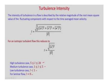
So, it is a some measure about the turbulence and you can see it is defined as the intensity of turbulence in a flow is described by the relative magnitude of the root mean square value of the fluctuating components with respect to the time average mean velocity. So, if I is the turbulent intensity, then it is root mean square value of this fluctuating component.
