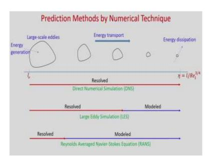
So, here you can see as we discussed you have a large scale eddies let us say its scale is of the order of l. So, it contains bulk kinetic energy due to the inertial effect it will be transported and due to the during the transport it will divide into smaller eddies.
