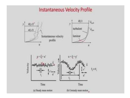
Here you can see the instantaneous velocity profile. So, velocity will vary with time . So, these are the velocity profile over a flat plate and if you time average the quantity then you will get this dotted line.
