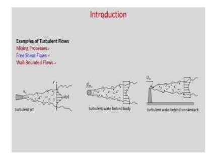
You can see examples of turbulent flows in mixing processes, free shear flows, wall bounded flows. So, these are some examples you can see in turbulent jet turbulent wake behind a body.
