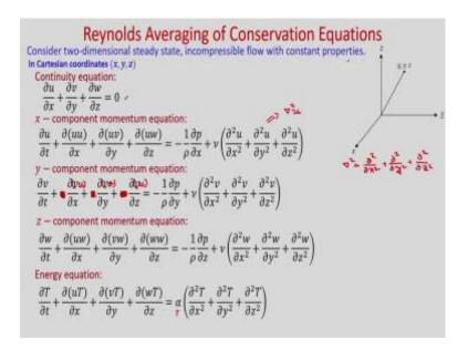
So, now these properties we can use for the when we will decompose the velocities and temperature into mean quantity and the fluctuating component. So, first we will start with the Navier stokes equations, we will write the Navier stokes equation in weak conservative form. So, you can see if you consider two dimensional steady state incompressible flow with constant properties.
