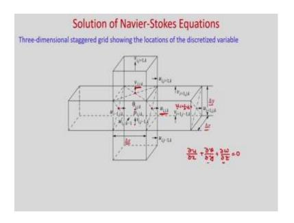
So, now let us see the cell, where we need to discretize the continuity equation as well as the energy equation. And the staggered grid where we need to solve the velocities. So, we can see this is the main cell, where at center you will solve for P and this cell is i j k index is i j k, and we need to solve for temperature, so,  $t_{i,j,k}$  or  $\theta_{i,j,k}$ , where  $\theta$  is non-dimensional temperature.
