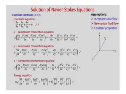
So, let us consider these equations in Cartesian coordinate. So, for incompressible Newtonian fluid flow with constant properties, this is the continuity equation. This is the x component of momentum equation, and this is y component of momentum equation, and this is the energy equation. In today's class we will just discretize the Navier-Stoke equations and you can see how many variables are there? u, v, w, p,. And if you solve for energy then will be temperature.
