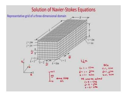
So, you know that first we need to discretize the domain into grids so, that we can solve the discretized equation in a discrete point. So, if you consider this three-dimensional domain. And you can see this is divided into grid x direction is in these direction, this is the y direction, and this is the z direction and the grid we are giving the index with i, j, and k. So, you can see this is your j = 1 and it is varying in this direction and it is j = j i m and previous cell is j r e.
