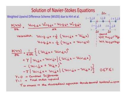
So, this is the scheme we will use weighted upwind difference scheme, which is known as WUDS due to Hirt et. al. So, you can see we have  $\frac{\partial (uu)}{\partial x}$ . So, what we will see so, this is to be discretized for the velocity here i,j,k. So, we will use  $\frac{\partial (uu)}{\partial x} = \frac{u_{i+\frac{1}{2},j,k}u_{i+\frac{1}{2},j,k}^* - u_{i-\frac{1}{2},j,k}u_{i-\frac{1}{2},j,k}^*}{\Delta x}$ .
