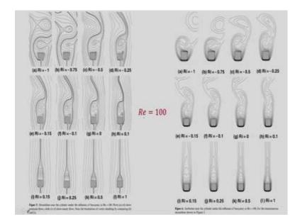
So, you can see that for Reynolds number 100, and Prandtl number is 0.7. You can see the flow physics. These are the streamlines near the cylinder under the influence of buoyancy. So, you can see these cases are from Richardson number 0.15 to 1, you can see you have a steady flow.
