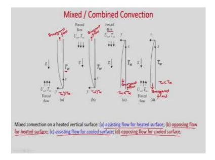
So, if you consider only flow over vertical plate, you can define the assisting or opposing flow for different thermal conditions. So, you can see in this case if it is heated surface, so  $T_w > T_\infty$  in obviously, if it is forced flow direction in upward direction, then it is a assisting flow for heated surface.
