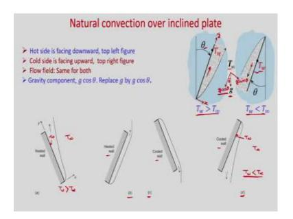
So, you can see in this case, say if it is an inclined plate where  $\theta$  is measured from the vertical line and  $T_w$  is the wall temperature and ambient temperature is  $T_\infty$ , and gravity is acting in negative y-direction. And if  $T_w > T_\infty$ , that means, your wall is maintained at higher temperature than the ambient temperature, then obviously, you will get this
