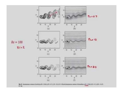
Now, you can see instantaneous contours of verticity, this left side figures; and in right side figure instantaneous contours of streamlines at Ri=2. So, this is Ri=2, Reynolds number 100, and for different Prandtl number . So, Prandtl number is 0.7, this is your Pr=10, and this is for Pr=80. So, you can see the effect of buoyancy .
