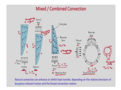
So, you can see here this particular case, you have a hot plate. And from the bottom, you are giving a forced flow. You have a fan; and from the fan this flow is going up. And buoyancy g is acting in this direction, and obviously, you can see buoyancy effect will be in this direction. Buoyancy emotion will be in this direction.
