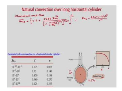
Now, let us consider flow over a horizontal circular cylinder. So, you can see this is the horizontal circular cylinder, where wall temperature is  $T_w$ , and ambient temperature is  $T_\infty$ . In this case,  $T_w > T_\infty$ . So, obviously, you can see boundary layer will be developed over this cylinder surface. And due to buoyancy effect, it will go up. And this lighter fluid will go up.
