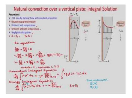
So, let us consider natural convection over a vertical flat plate. The plate is maintained at uniform wall temperature  $T_w$  and the quiescent medium temperature is  $T_\infty$  and that is also maintained at constant temperature. Here, we have these assumptions 2 dimensional steady laminar flow with constant properties, we have Boussinesq approximation valid and  $T_w$  is constant,  $T_\infty$  is constant and we are neglecting the viscous dissipation.
