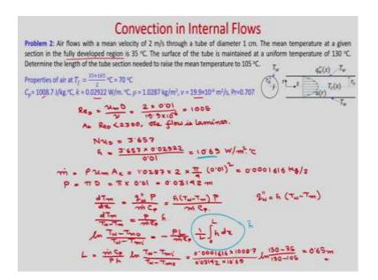
So, let us take the next problem; Air flows with a mean velocity of 2 m/s through a tube of diameter 1 cm. The mean temperature of a given section in the fully developed region is 35  $^{0}$ C.
