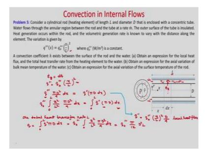
So, now we will consider this problem; Consider a cylindrical rod heating element of length L and diameter D that is enclosed with a concentric tube. Water flows through the annular region between the rod and the tube, at a rate m dot the outer surface of the tube is insulated heat generation occurs within the rod. And the volumetric generation rate is known to vary with a distance along the element. The variation is given by this relation.
