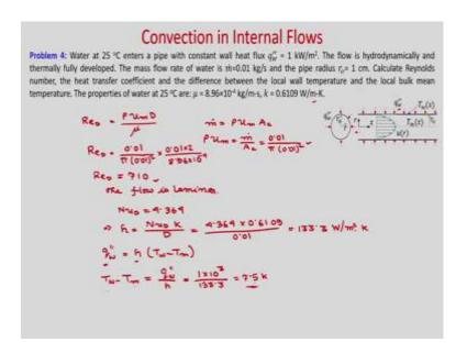
So, let us discuss about this problem; Water at 25  $^{0}$ C enters a pipe with constant wall heat flux  $q_{w}^{"}=1$  kW/m<sup>2</sup>. The flow is hydro dynamically and thermally fully developed.
