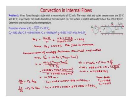
So, first let us take this problem; Water flows through a tube with a mean velocity of 0.2 m/s. The mean inlet and outlet temperatures are 20°C and 80 °C respectively. The inside diameter of the tube is 0.5 cm, the surface is heated with uniform heat flux of 0.6 W/cm². Determine the maximum surface temperature. So, you can see it is uniform wall heat flux boundary condition.
