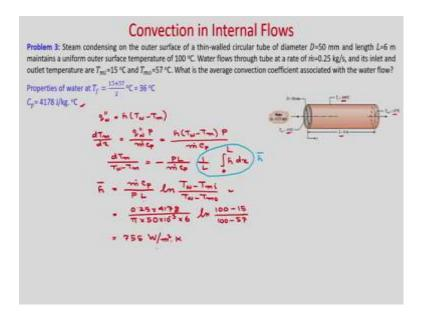
Let us discuss about the next problem; Steam condensing on the outer surface of a thin walled circular tube of diameter D = 50 mm and length L is 6 m, maintains a uniform outer surface temperature of  $100\,^{0}$ C, water flows through tube at a rate of m = 0.25 kg/s. And its inlet and outlet temperatures are  $15\,^{0}$ C and  $57\,^{0}$ C respectively. What is the average convection coefficient associated with the water flow?
