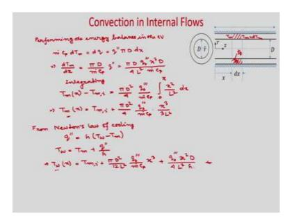
So, now you perform the energy balance in the control volume. So, performing the energy balance in the control volume. So, this is the control volume. So, whatever  $E_g$  is generated. So, dq is taken by the fluid. So, you can see you will get  $mC_p dT_m$  and  $dT_m$  is the change in the mean temperature.
