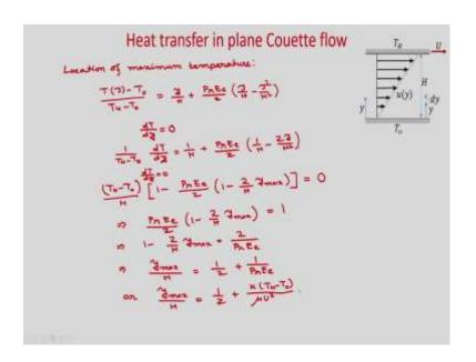
So, your temperature distribution, so location of maximum temperature. So, how we will find? So, let us see the temperature distribution  $\frac{T(y) - T_0}{T_H - T_0} = \frac{y}{H} + \frac{\Pr{Ec}}{2} \left( \frac{y}{H} - \frac{y^2}{H^2} \right).$
