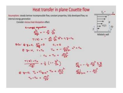
So, here we are considering  $T_H$  on the top wall and adiabatic wall on the bottom. So that means, there will be no heat transfer. So, in this particular case, if you see already we have derived the energy equation and your energy equation is energy equation already we have derived. So,  $\frac{d^2T}{dv^2} = -\frac{\mu}{K}\frac{U^2}{H^2}$ , we have consider the viscous dissipation effect.
