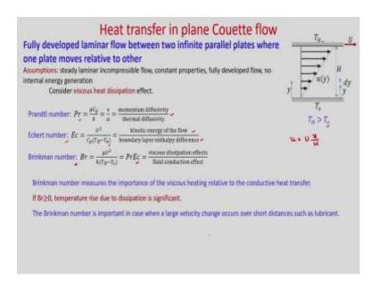
So, let us consider the flow between two parallel plates; the bottom plate here velocity is 0, so it is stationary plate and upper plate, you can see it is moving in the x direction with a constant velocity u. The bottom plate is maintained at temperature  $T_0$  and upper plate is maintained at temperature  $T_H$ , where  $T_H$  we are considering is greater than  $T_0$  and y is measured from the bottom wall and the distance between two plates is H.
