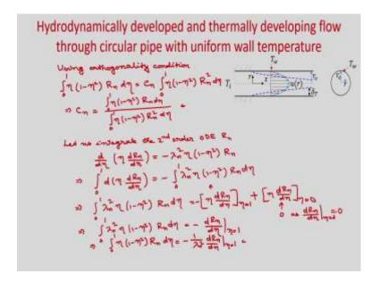
So, if you keep only n=m, then using orthogonality condition so, you can write  $\int_{0}^{1} \eta (1-\eta^2) R_n d\eta = \int_{0}^{1} \sum_{n=0}^{\infty} C_n \eta (1-\eta^2) R_n^2 d\eta$ .
