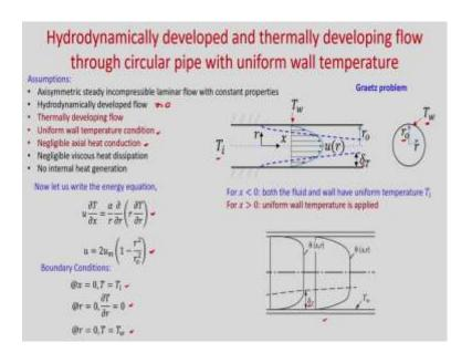
So, you can see that we are considering hydrodynamically developed and thermally developing; that means, you can see that your thermal boundary layer is growing. This is the thermal boundary layer thickness  $\delta_T$  and in developing region we need to find what is the temperature distribution.
