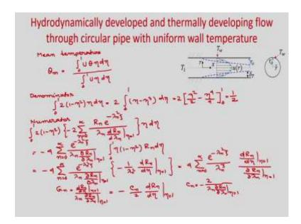
Now, we are interested to find the Nusselt number. So, to find the Nusselt number we have to find the difference we need to find the temperature difference between mean temperature and the wall temperature. So, for that first we need to find what is the mean temperature. So, you can see that bulk mean temperature mean
