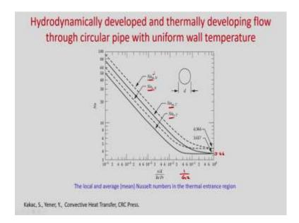
So, we can see the temperature profile. So, Nusselt number is plotted with  $\frac{x/d}{\text{Re}_D \text{Pr}}$  which
