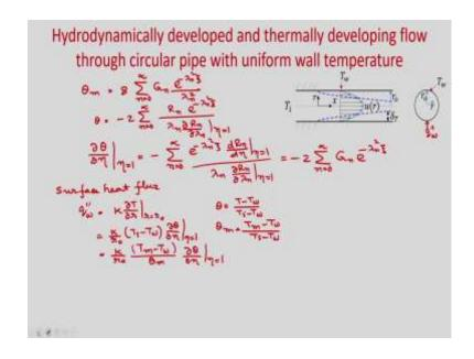
So, you will get the final expression for mean temperature  $\theta_m = 8 \sum_{n=0}^{\infty} G_n \frac{e^{-\lambda_n^2 \xi}}{\lambda_n^2}$ . So, now, to calculate the Nusselt number we need the temperature gradient at  $\eta = 1$ ; that means, at the wall. So, we need the temperature gradient at  $\eta = 1$ .
