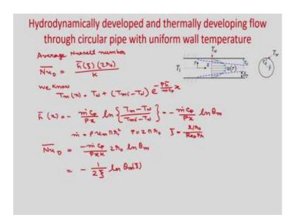
So, average Nusselt number if you calculate . So, you can write  $\overline{Nu_D} = \frac{\overline{h}(\xi)(2r_0)}{K}$ . So, it will be and from the energy balance we know  $T_m(x) = T_w + (T_{mi} - T_w)e^{\frac{-\frac{P\overline{h}}{m}x}{mC_p}}$ .
