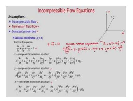
So, now, let us discuss some important governing equations in fluid mechanics. So, the main assumptions we are taking incompressible flow, Newtonian fluid flow and constant properties. So, in this case we are considering Cartesian coordinate. So, in x direction you have velocity u in y direction you have velocity v and in z direction you have velocity w.
