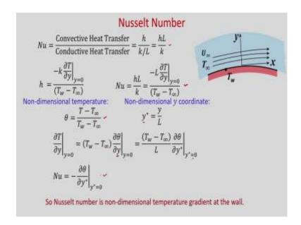
We have discussed about the heat transfer coefficient and very often we write this heat transfer in non-dimensional form and this non-dimensional number is known as Nusselt number. Nusselt number is the ratio of conductive to convective heat transfer in a fluid. So, you can see
