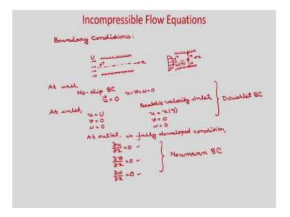
So, when you solve these equations you need to have the boundary conditions. So, if we discuss the boundary conditions for fluid flow. So, if you consider flow between parallel plates. So, these are the 2 parallel plates in third direction let us say it is infinite. So, you have fluid flow in axial direction x, this is your y and so obviously if these are walls then
