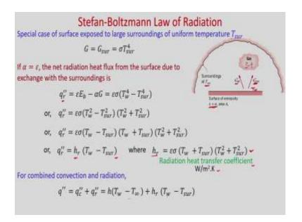
Now, let us consider a special case. Surface exposed to large surrounding to uniform temperature  $T_{sur}$ . So, you have the surface whose temperature is  $T_w$ . So, due to convection there will be heat flux  $q''_{conv}$ . Due to radiation there will be heat flux  $q''_{rad}$ . Your ambient temperature is  $T_{\infty}$  heat transfer coefficient is h; surrounding temperature is maintained at  $T_{sur}$ .
