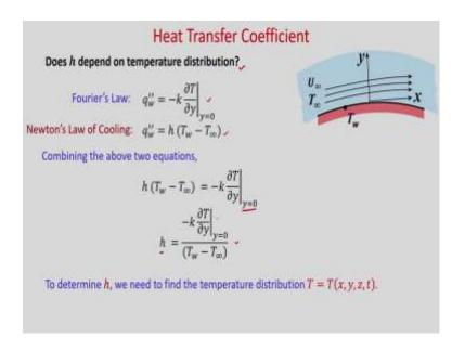
Now, the question is does h depend on temperature distribution. So, let us see in Fourier's law the heat flux at the wall we can write  $q'_{w} = -k \frac{\partial T}{\partial y}|_{y=0}$ . So, at the wall.
