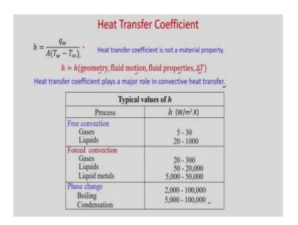
So, you can see heat transfer coefficient is the heat transfer rate per unit area per unit temperature difference. So, here you can see that heat transfer coefficient is not a material property. So, it is a transport property and it depends on many things. So, it depends on geometry, fluid motion, fluid properties and sometime on temperature difference. So, heat transfer coefficient plays a major role in convective heat transfer.
