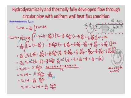
So, now let us calculate the mean temperature. So, that you can calculate  $T_m(x) = \frac{1}{m^A} \int \rho u T dA$ . So, if you consider this elemental flow area d A at a distance r of
