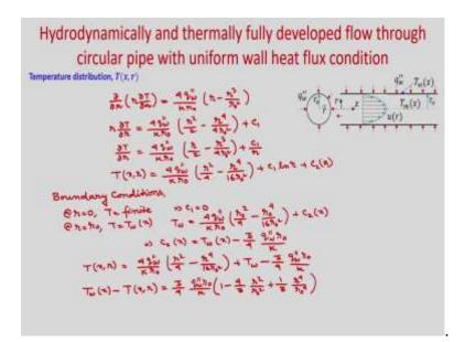
So, what is your equation finally we got? So, that is your  $\frac{\partial}{\partial r} \left( r \frac{\partial T}{\partial r} \right) = \frac{4q_w^2}{Kr_0} \left( r - \frac{r^3}{r_0^2} \right).$
