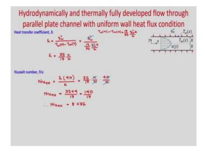
So, heat transfer coefficient will be. So, heat transfer coefficient is  $h = \frac{q_w}{T_w(x) - T_m(x)}$ . So,
