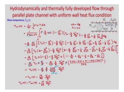
So, mean temperature you can find  $T_m(x) = \frac{1}{mA} \int_A \rho u T dA$ . So, if you consider from the centreline, one small elemental flow area of distance dy at a distance y from the centreline.
