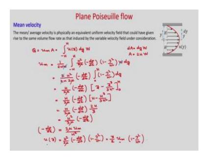
So, you can see that mean or average velocity is physically an equivalent uniform velocity field that could have given rise to the same volume flow rate as that induced by the variable velocity field under consideration. So, if you calculate the volume flow rate Q, so you can write  $Q = u_m A$ , where  $u_m$  is the mean velocity.
