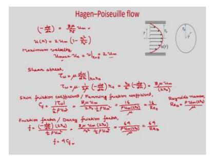
So,  $-\frac{dP}{dx}$  you can express in terms of mean velocity, so that will be  $-\frac{dP}{dx} = \frac{8\mu}{r_0^2} u_m$ . So, now, you can express this velocity profile in terms of the mean velocity. So, you can see that,  $u(\mathbf{r}) = 2u_m(1-\frac{r^2}{r_0^2})$ .
