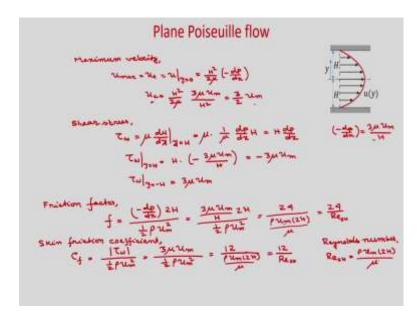
So, you will get maximum velocity. So, maximum velocity will occur at central line, where u at y =0. So, if you put it, you are going to get  $u_{max} = u_c = u \Big|_{y=0} = \frac{H^2}{2\mu} (-\frac{dP}{dx})$ . And that if you write  $-\frac{dP}{dx}$  in terms of  $\frac{3\mu u_m}{H^2}$ , then you are going to get,  $u_c = \frac{H^2}{2\mu} \frac{3\mu u_m}{H^2}$ .
