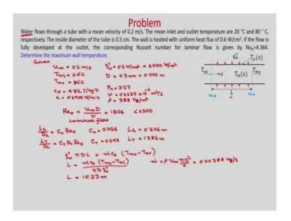
So, now let us solve one example problem; Water flows through a tube with a mean velocity of 0.2 m/s. The mean inlet and outlet temperature are 20°C and 80°C
