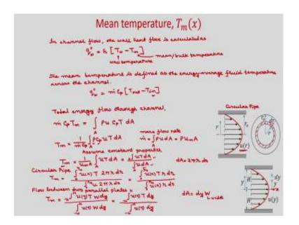
In external flow, we have seen that you can calculate the wall heat flux as  $q_w = h[T_w - T_m]$  which is your Newton's law of cooling. Here,  $T_w$  is the wall temperature and  $T_\infty$  is the free stream temperature. But, internal flows you can see that, there is no such free stream temperature.
