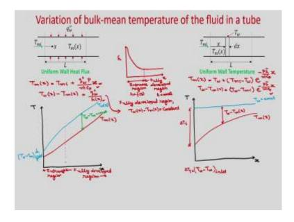
So, now for both the thermal conditions, we have found what is the axial variation of mean temperature as well as the total heat transfer rate. Now, let us see the variation of this bulk mean temperature of the fluid in the tube. So, you can see for uniform wall heat flux so, what is the variation of  $T_{\rm m}$ ?
