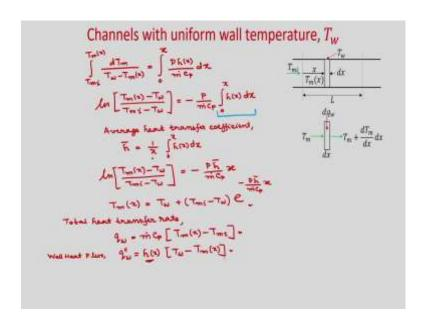
So, now, you integrate it from x =0 to any distance x so, if you do that. So, now, integrate this. So, from at x =0, you have  $T_{mi}$  and at any distance x, you have  $\int_{T_{mi}}^{T_m(x)} \frac{dT_m}{T_w - T_m(x)} = \int_0^x \frac{Ph(x)}{\dot{m}C_n} dx$ .
