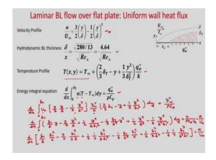
So, we can see we have the velocity profile already we have derived using third degree polynomial and from that solution, hydrodynamic boundary layer thickness we have found,  $\frac{\delta_T}{x}$  as this. In today's class we have found the temperature distribution for the given boundary conditions and this is the energy integral equation. So, now, you put the value of u here and value of T here; so you will be able to find, what is the thermal boundary layer thickness?
