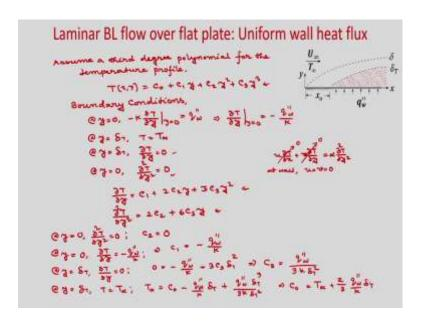
So, assume a third degree polynomial for the temperature profile. So, T which is function of (x, y) we can write  $T(x, y) = C_0 + C_1 y + C_2 y^2 + C_3 y^3$ . So, these coefficients  $Cc_0$ ,  $C_1$ ,  $C_2$ ,  $C_3$  are function of x. So, now, we have boundary conditions at y = 0; y = 0, you can see your heat flux is given. So, you can write  $-K \frac{\partial T}{\partial y} \Big|_{y=0} = q_w^{"}$ .
