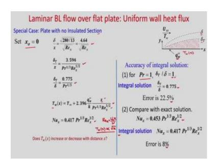
So, you can see in this particular case  $x_0=0$ ; so, thermal boundary layer thickness and hydrodynamic boundary layer thickness starts developing from x=0. So, in for the special case, in earlier expression if you put  $x_0=0$ , where you have plate with no insulated section; then, we have already found  $\frac{\delta}{x}$ , then this is your  $\frac{\delta_T}{x}$  putting  $x_0=0$  and  $\frac{\delta_T}{\delta}$ .
