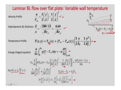
So, now we are considering laminar boundary layer flow over flat plate with variable wall temperature. So, you can see that your wall temperature varies with  $\sqrt{x}$ . So, we have taken this flat plate where temperature varies as  $T_{\infty} + C\sqrt{x}$ , where C is your constant.
