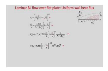
So, you can see, we have finally derived in today's class this  $\delta_T$  in terms of hydrodynamic boundary layer thickness  $\delta$ ; then putting the value of  $\delta$ , we have found  $\frac{\delta_T}{x}$ . And, you can see it is also function of Prandtl number and Reynolds number.
