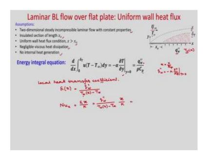
So, let us consider this flat plate, y is measured perpendicular to the flat plate, your free stream velocity is  $U_{\infty}$  and temperature is  $T_{\infty}$ . Up to  $x=x_0$  it is insulated, so it will be maintained at temperature  $T_{\infty}$  as there will be no heat transfer. From  $x=x_0$ , you can see this plate is maintained at uniform wall heat flux  $q_w^*$ .
