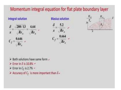
So you can see; finally, we have derived the hydrodynamic boundary layer thickness using integral solution  $\frac{\delta}{x} = \frac{4.64}{\sqrt{\text{Re}_x}}$ . Similarly, coefficient of friction we have derived
