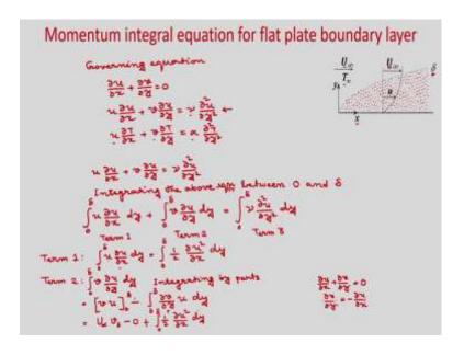
So now, let us consider flow over a heated flat plate. First, we will solve the fluid flow equation, then we will solve the energy equation for two different boundary conditions; with constant wall temperature and with constant heat flux.
