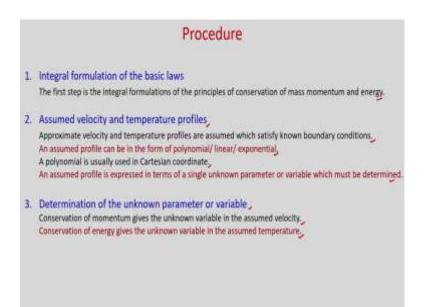
First, we have this integral formulation of the basic laws. The first step is the integral formulation of the principles of conservation of mass, momentum and energy. So, first you see, what are the governing equations for that fluid flow and heat transfer phenomena, then you write it in integral form.
