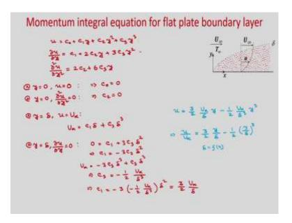
So, we have  $u = c_0 + c_1 y + c_2 y^2 + c_3 y^3$ . So  $\frac{\partial u}{\partial y}$ , if you take the derivative with respect to y. So you find the,  $\frac{\partial u}{\partial y} = c_1 + 2c_2 y + 3c_3 y^2$  and  $\frac{\partial^2 u}{\partial y^2} = 2c_2 + 6c_3 y$ .
