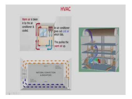
Now, we will discuss about the HVAC, Heating Ventilation and Air Conditioning. So, you can see the room where AC is there, so obviously this air condition gives out cold air and as it is cold air it is having high density. So, it will move inside the house and these pushes the warm air up.
