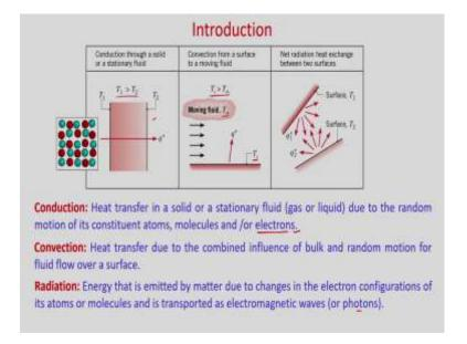
So, now let us define these three modes of heat transfer. Conduction: so, heat transfer in a solid or a stationary fluid gas or liquid takes place due to the random motion of its constituent atoms, molecules and or electrons.
