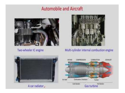
Now, let see some examples in automobiles and aircraft. You can see in your bike or two-wheeler. So, there will be IC engine, it has single cylinder and over it there will be some extended metal strip. So, those are known as fins. So, it increases the surface area and due to conduction from the cylinder surface actually, heat transfer takes place due to conduction. Inside the IC engine you know due to the combustion there will be high temperature and that is to be cooled.
