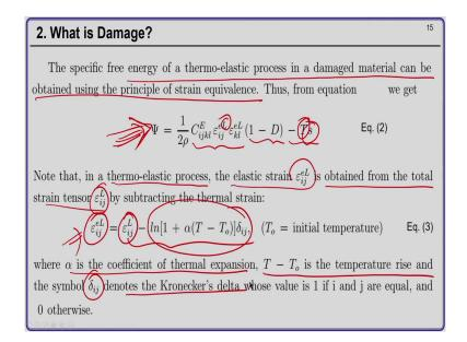
Now, the specific free energy of a thermo elastic process in a damaged material can be obtained using the principle of strain equivalence as follows, psi equal to 1 by 2 rho Cijkl epsilon ij epsilon kl and this L over here, denotes the logarithmic strain into 1 minus D minus T into s, where s is the specific entropy ok.
