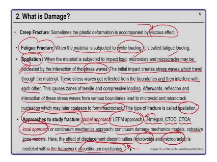
Now, we quickly look in to what is meant by creep fracture Ok. So, creep fracture is sometimes the plastic deformation is accompanied by viscous effect ok. So, in creep fracture you have to take into account viscous effect and in fatigue fracture the material is subjected to cyclic loading ok.
