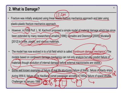
So, so, facture was initially analyzed using linear elastic fracture mechanics approach ok. And later on using the elasto-plastic fracture mechanics approach ok. So, the linear elastic fracture mechanics is called LEFM, this is still very popular where we find the stress intensity factor J integral and all these kind of concepts are there ok.
