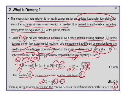
Now, this stress-strain relation is not convenient for the updated Lagrangian formulation and we will see what is meant by this for which the incremental stress strain relation is needed. So, it is derived in mathematical modeling starting with the expression 13 for the plastic potential.
