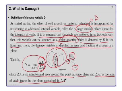
So, damage variable D is defined as follows. So, the effect of void growth on material behavior is incorporated by introducing an additional internal variable, called the damage variable, which is denoted as D which quantifies the intensity of the voids. If it is assumed that the voids are scattered in an isotropic way, then this variable can be assumed as a scalar quantity although people have used it as a tensor quantity also and this is denoted by D in the literature ok.
