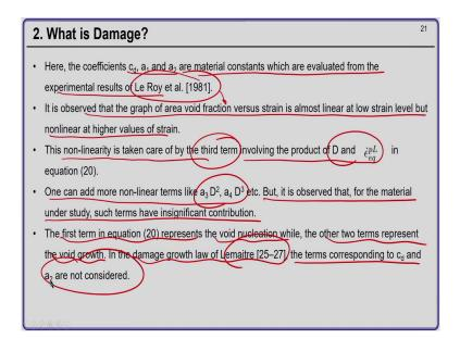
So, here the coefficients c d a 1 a 2 are material constant which are to be evaluated from the experimental results and for which we use the results of Le Roy and this we will discuss in the coming lectures. And, it is observed that the graph of area void fraction versus strain is almost linear at low strain level, but it is non-linearity higher values of strain ok.
