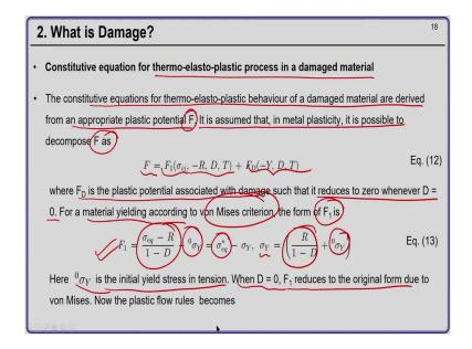
Now, the constitutive relation for a thermo elastoplastic process in a damaged material can be obtained as follows. So, the constitutive equation for the thermo elastoplastic behavior of a damaged material are derived from an appropriate plastic potential F. It is assumed that in metal plasticity it is possible to decompose F into 2 parts; one which is the plastic potential associated with the damage and one which is F 1 ok.
