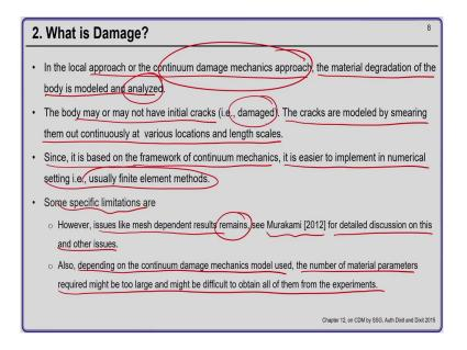
Now, in the local approach or the continuum damage mechanics approach which is what we will use in the formulation that will present the material degradation or the body is modeled ok.
