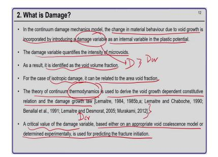
Now, in continuum damage mechanics model, the change in the material behavior is due to the void growth and it is incorporated by introducing a new variable which is called the damage variable. In our coming slides we will see what is meant by this damage variable, which is an internal variable in the plastic potential.
