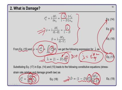
So, with this the plastic flow rule then can be written as following equation, where we have to find out this lambda star ok. So, here ok from equation number 15 which is here and this P, which can be identified with the equivalent plastic strain inside the body given by integral
