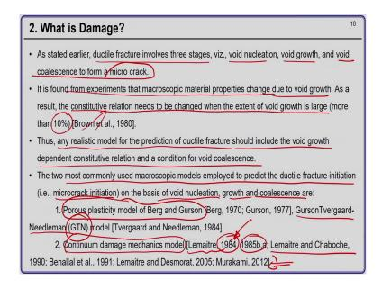
Now, as stated earlier ductile fracture involves three stages void nucleation, void growth, and void coalescence to form a micro crack. And, it is found from a experiments that macroscopic material properties change due to void growth ok.
