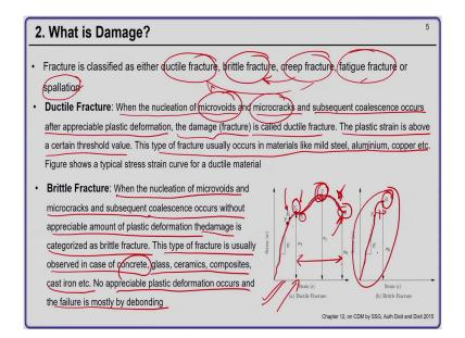
Now, fracture can be classified into what is called the ductile fracture, the brittle fracture, creep fracture, fatigue fracture and spallation ok. So, although these three can be categorized into either of these two, we have kept in separate and we just call them 5 different cases ok. So, ductile fracture is when the nucleation of microvoids and microcracks and subsequent coalescence occurs after appreciable plastic deformation.
