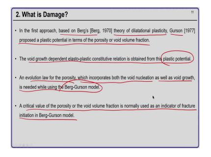
So, in the first approach which is based on the bergs theory of dilatational plasticity, Gurson proposed a plastic potential in terms of porosity or void volume fraction. And, the void growth dependent elastoplastic constitutive relation is obtained from this particular plastic potential ok. So, an evolution law for the porosity, which incorporates both the void nucleation as well as void growth is needed when you are using the Berg and Gursons model.
