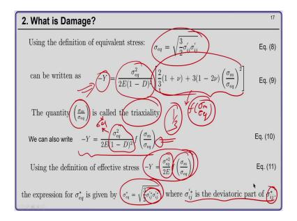
And, using the concept of equivalence stress ok, I can write minus Y ok. The dissipative part of Y as sigma equivalence square divided by 2 into 1 minus D square into this function. And, this function can be written as function of sigma m by sigma equivalent, where sigma ratio of sigma m the mean stress by equivalence stress is called triaxiality ok.
