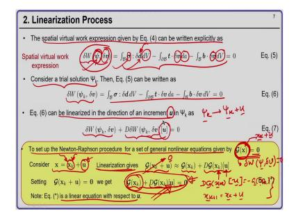
So, the spatial virtual work expression which is given by equation 4 can be written explicitly as, ok. So, now, I can write explicitly the virtual work as a function of the mapping psi in the virtual velocities, ok. So, psi is hidden somewhere here, in sigma and d, ok.
