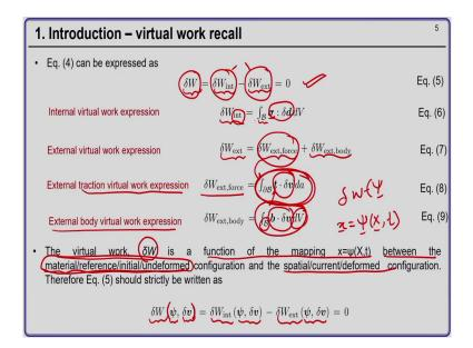
Now, equation 4 can be expressed as the difference of the virtual work of the internal forces and the virtual work of the external forces, ok. So, the total virtual work is nothing, but the difference of the internal virtual work and the external virtual work, and that should be equal to 0. So, in a way the at equilibrium the internal and external virtual work will balance out each other, ok.
