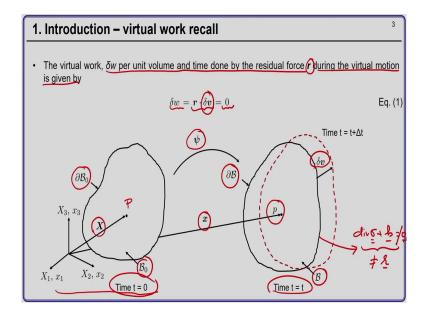
So, we first recall our derivation of virtual work expression, ok. So, in the figure as you see here you have a body in the initial configuration at time 0, ok. So, the configuration is B 0 and the surface of the body is del B 0.
