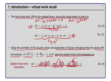
So, the total virtual work, that is del capital W by the residual forces r during the virtual motion will be given by del W equal to integral over the current volume r dot del v dV equal to 0, ok. So, del W, del capital W is nothing, but integral over the volume del w dV, ok, nd that should be equal to 0. So, when we substitute r as divergence of sigma plus p we get the total virtual work by the body forces as given by equation number 2, ok.
