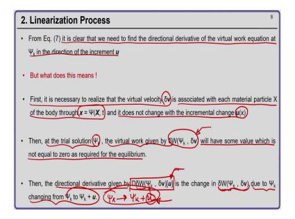
Now, let us think, more into it, ok. So, equation 7, it is clear that we need to find the directional derivative of the virtual work equation at psi k in the direction of the increment u to setup the Newton-Raphson iterative procedure. So, what does this actually means? We have to step back and pause for a moment and we have to ask what does directional derivative of the virtual work, equation at the trial solutions psi k in the direction of the increment u actually means, ok.
