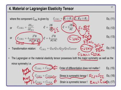
So, what will be C IJKL? C IJKL you can obtain and when we are discussing how to get the component of a fourth order tensor, this can be obtained by taking the double contraction of C with respect to E k, E L, E K tensor product E L and then, taking the double contraction of the resulting second order tensor with E I tensor product E J.
