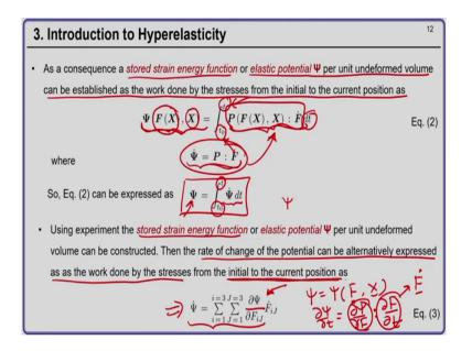
So, as a consequence of this, the stored energy strain energy function or the elastic potential psi per unit the undeformed volume can be established as a work done by the stresses from the initial to the current position as psi equal to P double contracted with the rate of deformation gradient tensor integrated over time from initial time to the current time.
