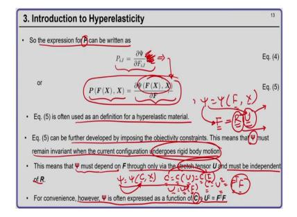
Now, the expression for the first Piola-Kirchhoff stress tensor can now be written as P equal to del psi by del F into F dot. So, as a direct notation, I can write P equal to del psi by del F sorry this will not be here, del psi by del F ok. So, this relation equation number 5 is used as a definition of hyper-elastic material. So, you can further develop equation 5, now using the objectivity constraints.
