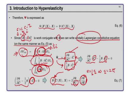
Therefore, psi which is has to be a function of deformation gradient tensor in the current position has to be a function of right Cauchy-Green tensor and the current position. Now, we know that the material time derivative of the Green-Lagrange strain tensor is twice the material time derivative of the right Cauchy-Green tensor.
