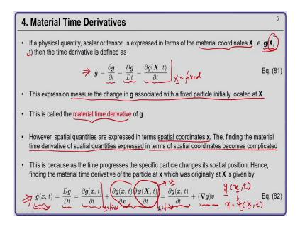
So, when a physical quantity ok; so any physical quantity for example, scalar or a tensor like temperature, velocity, stress, when they are expressed in terms of material coordinates X; that is g equal to X comma t ok. So, g can be scalar, g can be vector, g can be tensor, or any other higher order tensor.
