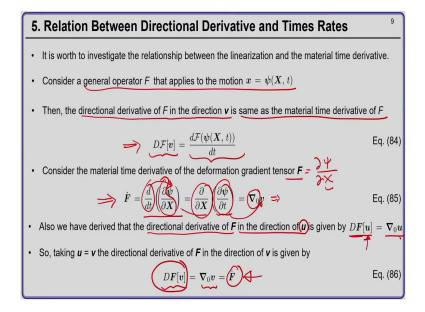
Now, there is a definite relation which exists between the directional derivative and the material time derivative ok. So, consider you have a general operator F that applies to the motion given by x equal to psi of X comma t.
