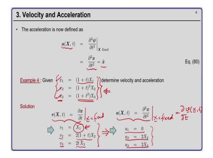
Now, moving on to acceleration. So, acceleration is now defined as the double derivative of the motion psi and its given by a equal to del square x by del t square or equal to x double dot ok. So, this equation number 80 gives you the current acceleration of a material particle which was located at material coordinate x. So, with this now let us take one example ok.
